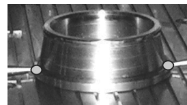
Fig. 6. Photography of the measurement of diameter of the big flange [D] made by MT_3 tool
