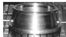
Fig. 7. Photography of the measurement of diameter of bearing way near the big flange [D 2 ] made by MT_3 tool
