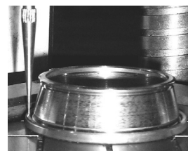
Fig. 8. Photography of the measurement of height of ancillary bearing way [a] made by MT_1 tool
