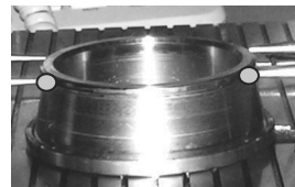
Fig. 5. Photography of the measurement of diameter of bearing way near the small flange [D 3 ] made by MT_3 tool
