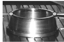
Fig. 4. Photography of the measurement of diameter of the small flange [D 1 ] made by MT_3 tool
