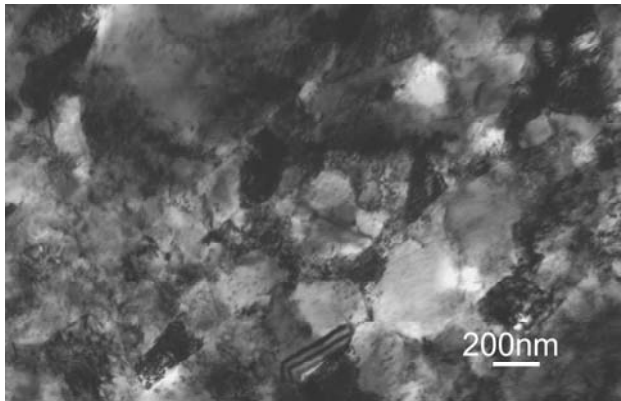
Fig. 20. Microstructure of copper after the ECAP 16 routes ( \phi = 18.4 ), (TEM)
