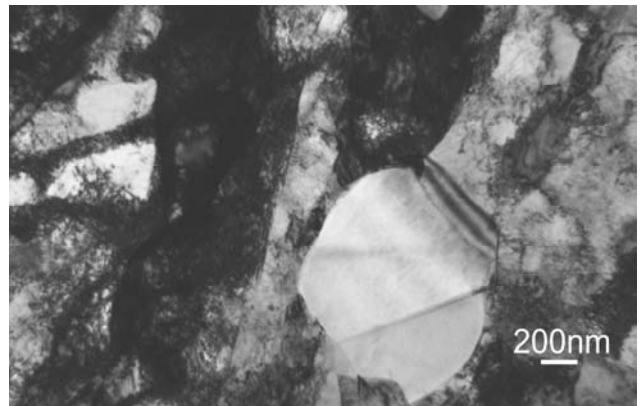
Fig. 17. Microstructure of copper after the combined deformation, 30 CEC cycles ( \varphi = 12.6 ) and HE ( \varphi = 1.83 ), (TEM)
