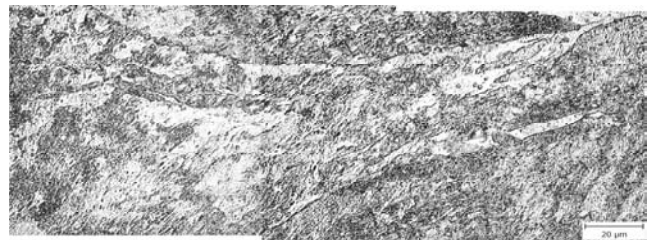
Fig. 3. Microstructure after 20 CEC cycles, \varphi = 17.9 , (MO)
