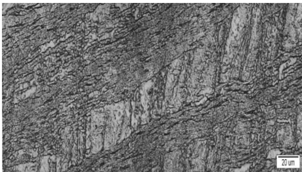
Fig. 5. Microstructure of copper deformed in the 4 ECAP routs ( \varphi = 4.6 ), (MO)
