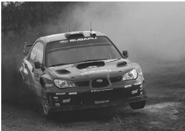
Fig. 6. Phenomenon of losing contact with the ground by front internal wheel. Picture from collection Subaru World Rally Team, presented here with approval from Subaru Import Polska Sp. z o.o.
