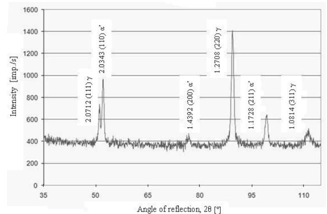
Fig. 10. X-ray diffraction patterns of X5CrNi18-8 steel after 43% of plastic deformation with and heat treatment at 500°C
