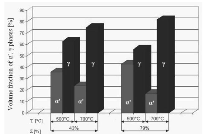
Fig. 11. Volume fraction of  $\gamma$  and  $\alpha'$  phases in structure of X5CrNi18-8 steel after cold deformation ( $Z$ ) and heat treatment at 500°C and 700°C ( $T$ )
