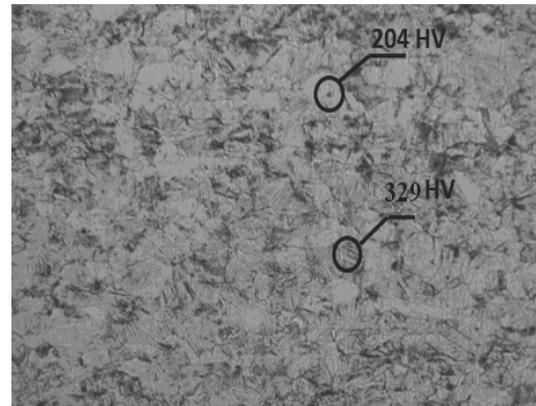
Fig. 3. Deformed austenite grains and  $\alpha'$  phase in the structure of X5CrNi18-8 steel cold rolled with 43% deformation degree and heat-treated at 550°C; Mag. 200x
