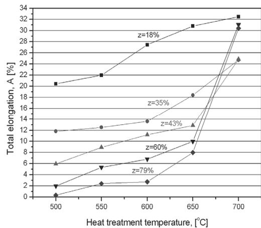
Fig. 8. The influence of the heat treatment temperature and degree of cold deformation ( $z$ ) on the values of  $A$
