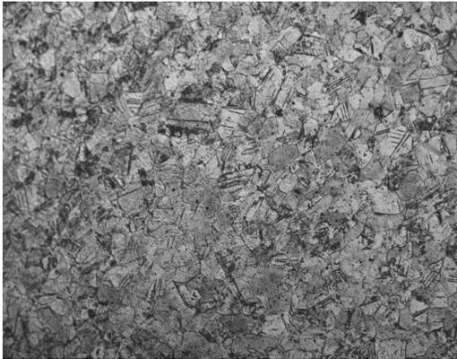
Fig. 1. Structure of the investigated steel after 18% of plastic deformation; Mag. 200x
