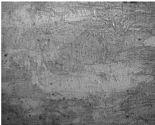
Fig. 2. Deformed austenite grains and  $\alpha'$  phase in the structure of X5CrNi18-8 steel cold rolled with 79% deformation degree; Mag. 500x
