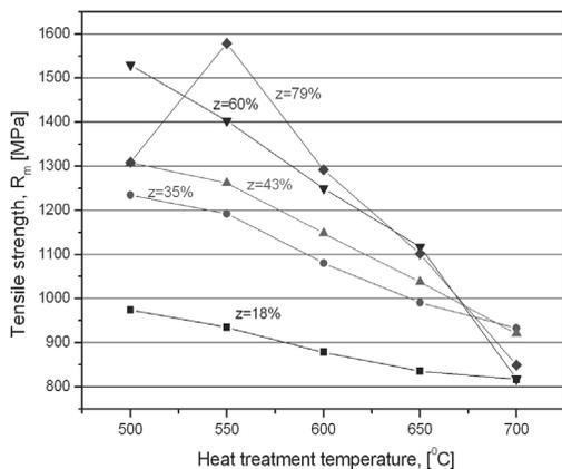
Fig. 6. The influence of the heat treatment temperature and degree of cold deformation ( $z$ ) on the values of  $R_m$
