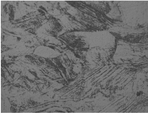
Fig. 5. Austenite grains with slip bands and  $\alpha'$  phase in the structure of X5CrNi18-8 steel cold rolled with 43% deformation degree and heat-treated at 600°C; higher magnification of the  $\alpha'$  phase shown in Fig. 4; Mag. 1000x
