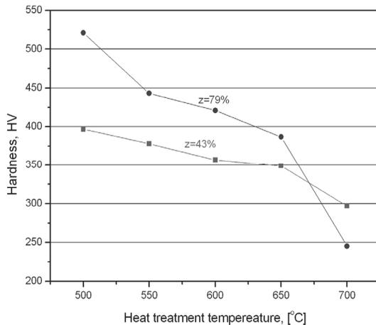
Fig. 9. The influence of the heat treatment temperature and degree of cold deformation ( $z$ ) on the values of  $HV$
