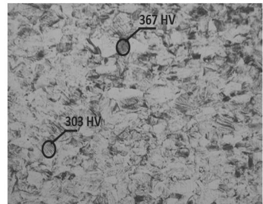
Fig. 4. Deformed austenite grains and  $\alpha'$  phase in the structure of X5CrNi18-8 steel cold rolled with 43% deformation degree and heat-treated at 600°C; Mag. 200x
