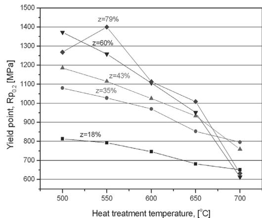
Fig. 7. The influence of the heat treatment temperature and degree of cold deformation ( $z$ ) on the values of  $R_{p0.2}$
