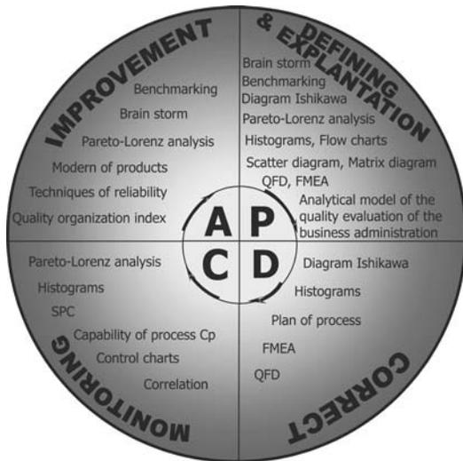
Fig. 1. Model PDCA connects with quality methods and quality tools [7]
