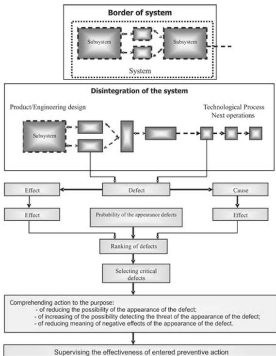
Fig. 6. Stages of FMEA method [20]
