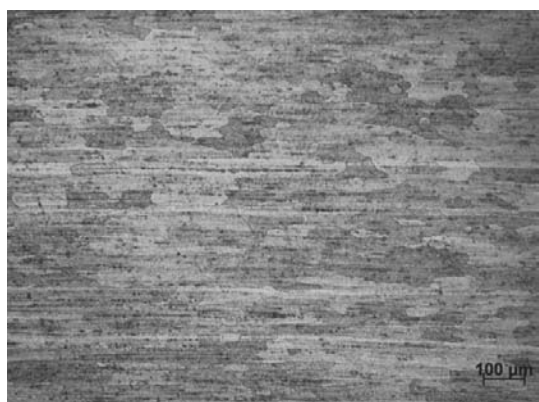
Fig. 3. Matrix - \alpha with fine precipitations. AlMg1.5 alloy after supersaturation
