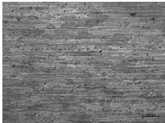
Fig. 5. Grains of the \alpha - solution with precipitations. AlMg3.5Mn alloy after supersaturation
