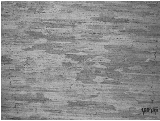
Fig. 7. Grains of the \alpha - solution with precipitations arranged in bands. AlMg1.5 alloy after CHT, ageing at 200°C
