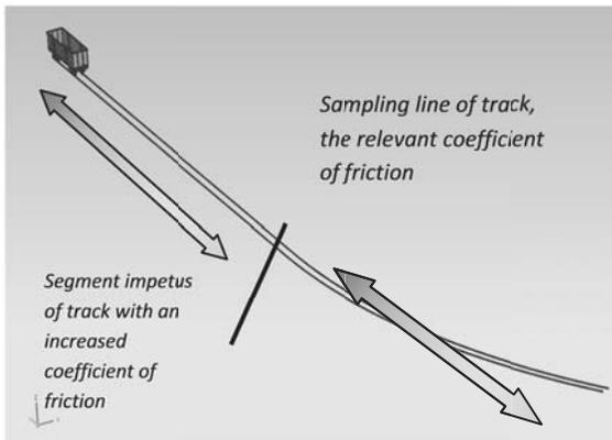
Fig. 6. Movement of a wagon variant used in the work
