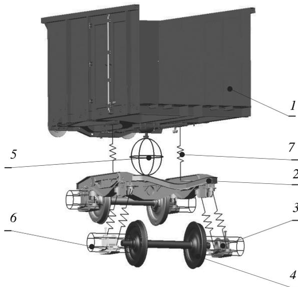
Fig. 5. Referential diagram: 1 - link box, 2 - link carriage, 3 - link socket bearings, 4 - link wheel set, 5 - joint spherical, 6 - joint revolute, 7 - connector spring
