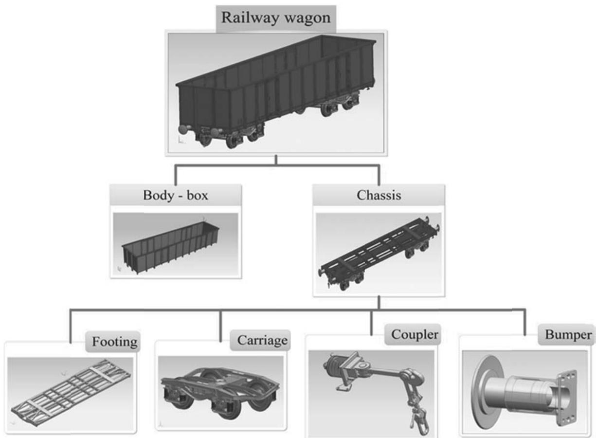
Fig. 1. Diagram of the railway wagon
