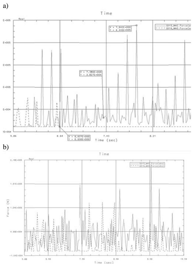
Fig. 8. A chart comparing the pressure forces inner and outer wheels single axes for speeds of: a) 130 km/h, b) 90 km/h. The red graph symbolizes the outer wheel, blue graph inner wheel
