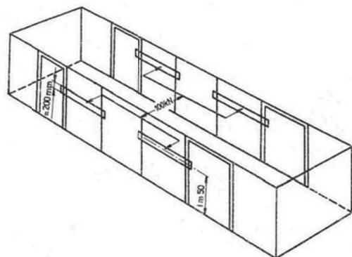
Fig. 4. Strength test of the side walls of the wagon [1-3]
