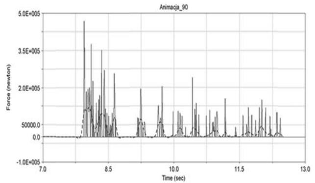
Fig. 11. Graph of pressure force between wheels and rail at speed of 90 km/h
