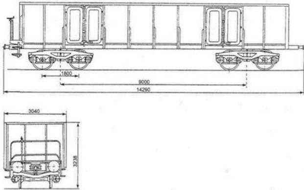
Fig. 2. Overall dimensions of the railway wagon [13]
