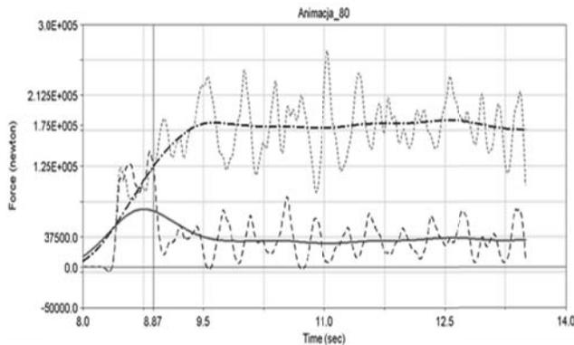
Fig. 13. Graph of pressure force the inside wheel (blue) and external (pink), red and dark blue lines are the averaged values of pressure at individual wheels
