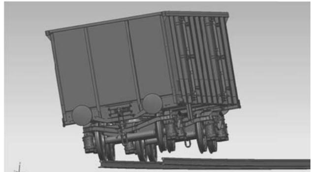
Fig. 7. View heeling a car at a speed of 130 km/h
