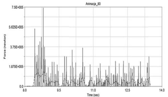
Fig. 12. Graph of pressure force between wheels and rail at speed of 80 km/h
