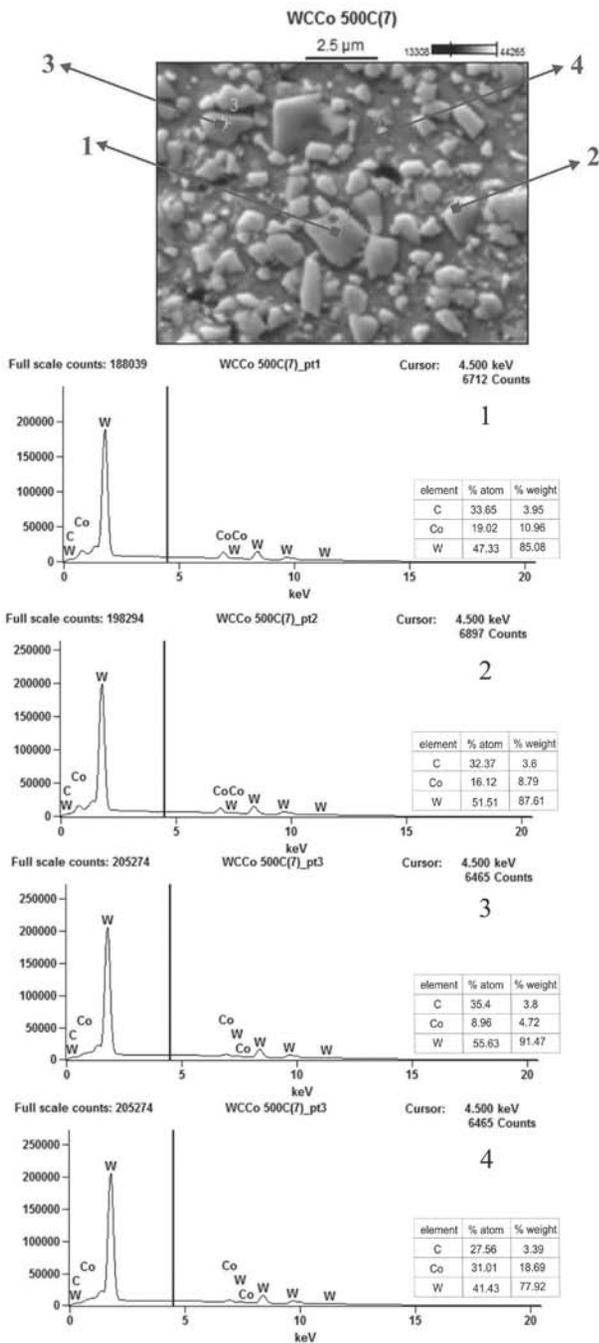
Fig. 11. Microstructure and chemical composition of the HVOF sprayed WC-Co coating and annealed at the conditions: T = 500°C, t = 24 h
