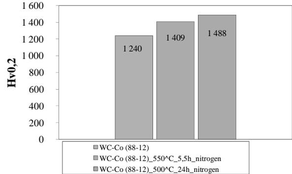
Fig. 12. Microhardness of the HVOF sprayed WC - Co coating and annealed in the different conditions
