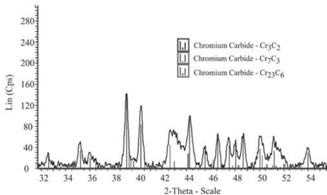
Fig. 7. Phase composition of  $\text{Cr}_3\text{C}_2\text{-NiCr}$  coating
