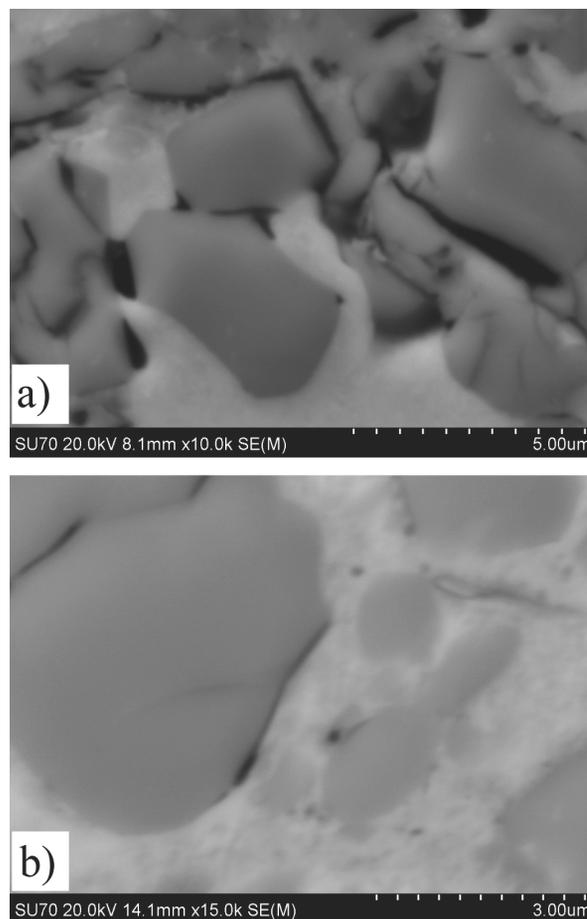
Fig. 2. Cracks localized in the neighbourhood of the carbides in the HVOF sprayed  $\text{Cr}_3\text{C}_2\text{-NiCr}$  coatings; a) HVOF sprayed, b) HVOF sprayed and annealed at the conditions:  $T = 550^\circ\text{C}$ ,  $t = 5.5$  h
