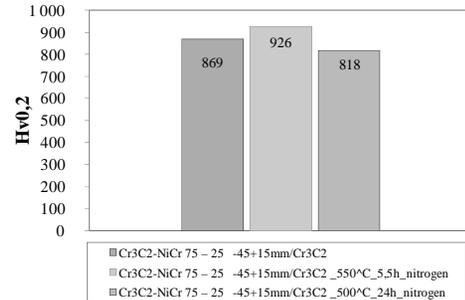
Fig. 8. Microhardness of the HVOF sprayed  $\text{Cr}_3\text{C}_2\text{-NiCr}$  coating and annealed in the different conditions
