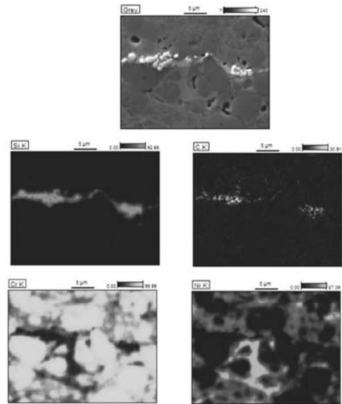
Fig. 4. Microstructure of the HVOF sprayed  $\text{Cr}_3\text{C}_2\text{-NiCr}$  coating and then annealing at the conditions:  $T = 500^\circ\text{C}$ ,  $t = 24$  h with maps of the elements distributions
