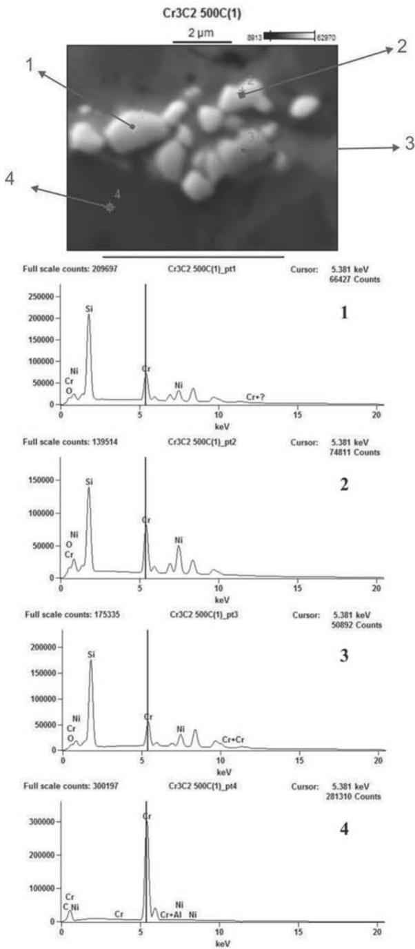
Fig. 3. Microstructure and chemical composition of the particles presented in the HVOF sprayed  $\text{Cr}_3\text{C}_2\text{-NiCr}$  coating and annealed at the conditions:  $T = 500^\circ\text{C}$ ,  $t = 24$  h
