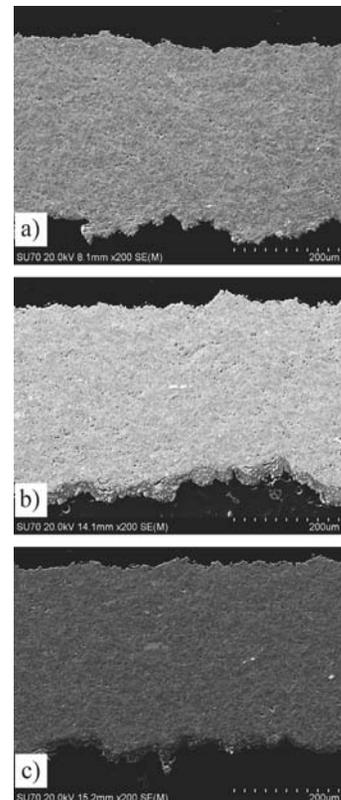
Fig. 5. Cross section of the HVOF sprayed  $\text{Cr}_3\text{C}_2\text{-NiCr}$  coating; a) HVOF sprayed, b) HVOF sprayed and annealed at the conditions:  $T = 550^\circ\text{C}$ ,  $t = 5.5$  h, c) HVOF sprayed and annealed at the conditions:  $T = 500^\circ\text{C}$ ,  $t = 24$  h
