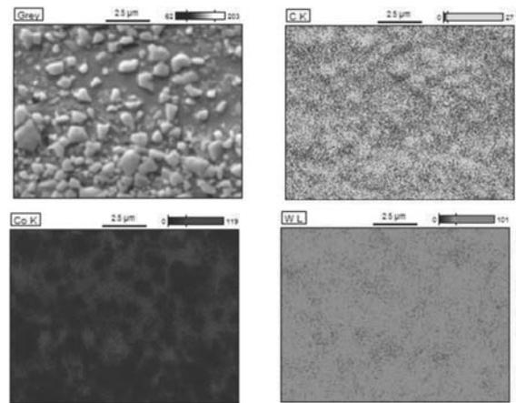
Fig. 10. Microstructure of the HVOF sprayed WC-Co coating and then annealing at the conditions:  $T = 500^{\circ}\text{C}$ ,  $t = 24$  h with maps of the chemical elements distributions
