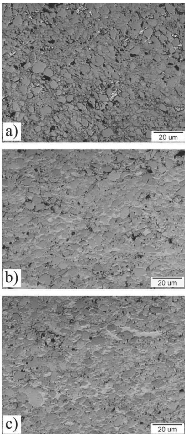
Fig. 1. Microstructures of the HVOF sprayed  $\text{Cr}_3\text{C}_2\text{-NiCr}$  coatings; a) HVOF sprayed, b) HVOF sprayed and annealed at the conditions:  $T = 550^\circ\text{C}$ ,  $t = 5.5$  h, c) HVOF sprayed and annealed at the conditions:  $T = 500^\circ\text{C}$ ,  $t = 24$  h
