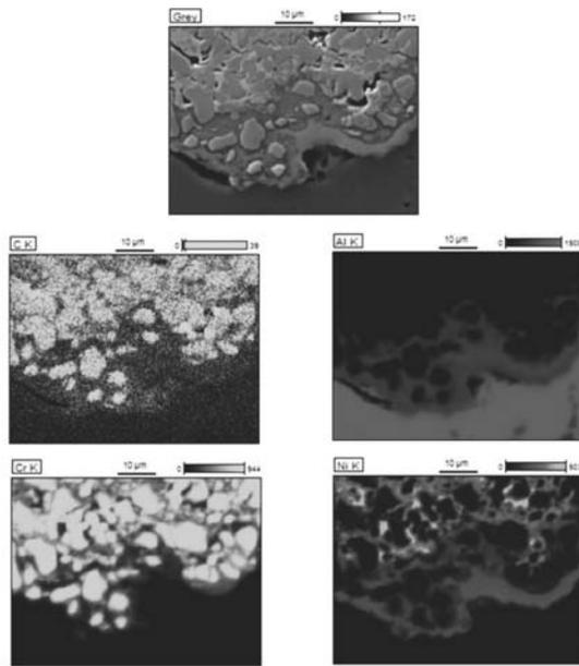
Fig. 6. Microstructure of the HVOF sprayed  $\text{Cr}_3\text{C}_2\text{-NiCr}$  coating and then annealing at the conditions:  $T = 500^\circ\text{C}$ ,  $t = 24$  h with maps of the elements distributions on the contact layer - substrate
