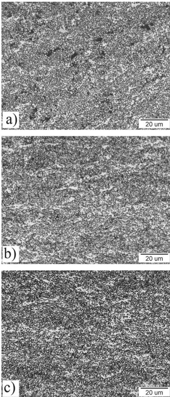
Fig. 9. Microstructures of the HVOF sprayed WC-Co coatings; a) HVOF sprayed, b) HVOF sprayed and annealed at the conditions:  $T = 550^{\circ}\text{C}$ ,  $t = 5.5$  h, c) HVOF sprayed and annealed at the conditions:  $T = 500^{\circ}\text{C}$ ,  $t = 24$  h
