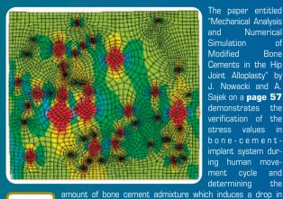
The paper entitled "Mechanical Analysis and Numerical Simulation of Bone Modified Cements in the Hip Joint Alloplasty" by J. Nowacki and A. Sajek on a page 57 demonstrates the verification of the stress values in bone-cementimplant system during human moveand determining the
