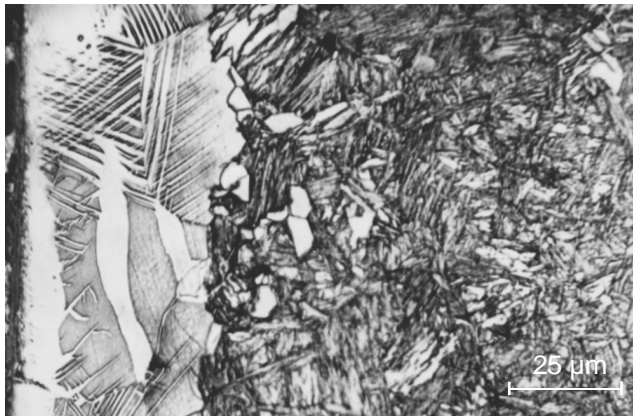
Fig. 8. Surface layer microstructure of 38CrAlMo6-10 steel quenched from 920°C, tempered at 575°C and gas-nitrided at 570°C for 8 hrs in an ammonia atmosphere
