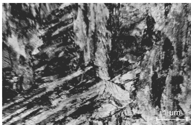
Fig. 24. Microstructure of X37CrMoV5-1 steel quenched from 1030°C and tempered at 600°C; thin foil
