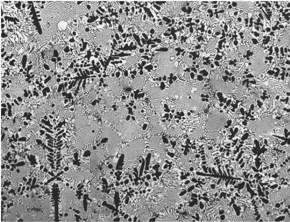
Fig. 8. Microstructure of the ZL8 cast alloy, modified with 0.5% (mass) La and 0.5% (mass) Ce etched in 10% HF, mag. 100x
