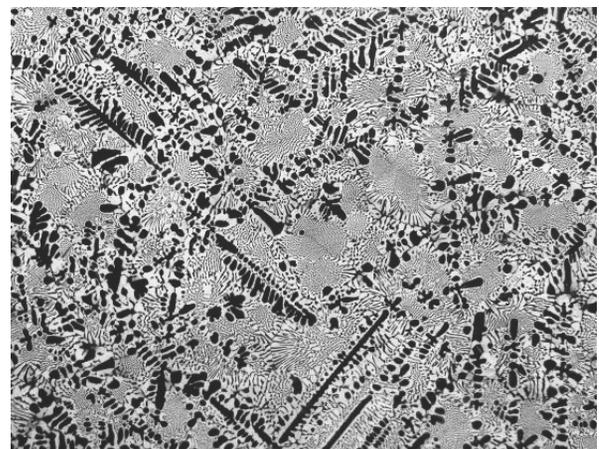
Fig. 6. Microstructure of the non-modified ZL8 cast alloy, etched in 10% HF, mag. 100x
