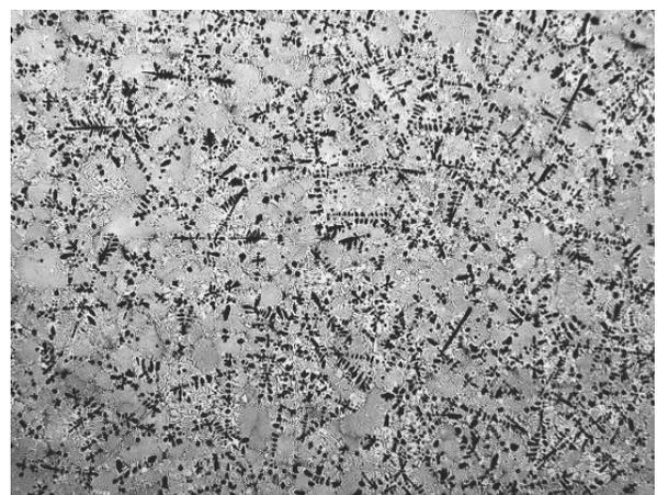
Fig. 7. Microstructure of the ZL8 cast alloy, modified with 0.5% (mass) La and 0.5% (mass) Ce etched in 10% HF, mag. 25x
