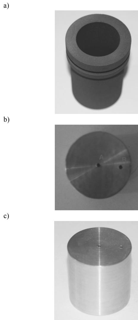
Fig. 1. Elements of the investigation configuration: a) graphite crucible, b) and c) sample
