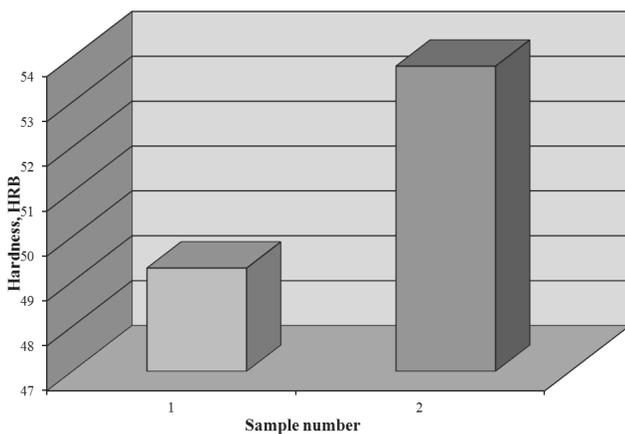
Fig. 9. Hardness measurement results of the ZL8 alloy: 1 - non-modified, 2 - modified with La and Ce
