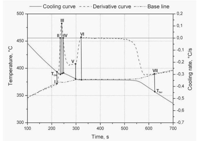
Fig. 2. Cooling curve, crystallisation curve and calorimetric analysis of the ATD diagram for the ZL8 alloy, cooling rate 0.09°C/s
