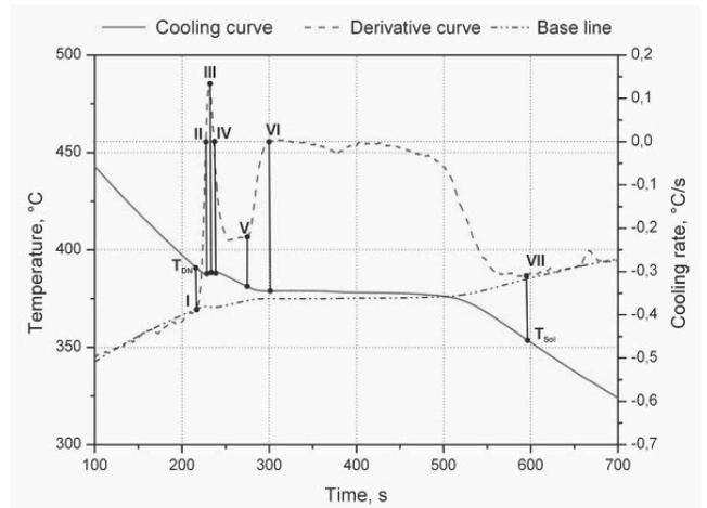
Fig. 3. Cooling curve, crystallisation curve and calorimetric analysis of the ATD diagram for the ZL8 alloy, modified with 0.5% (mass) La and 0.5% mass Ce cooling rate 0.15°C/s
