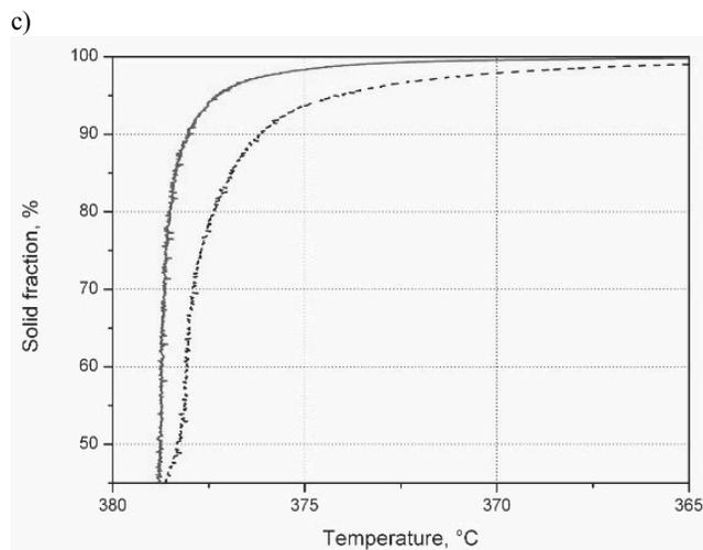
Fig. 4. Fraction solid diagram of the ZL8 alloy: a) entire diagram, b) and c) magnified part of the diagram from Fig. 4a
