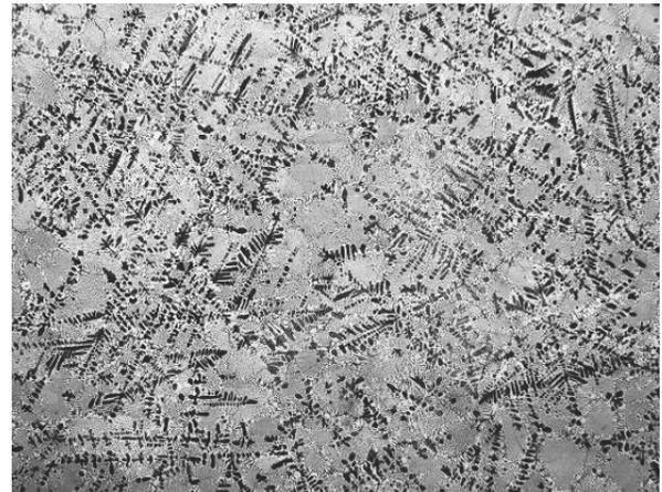
Fig. 5. Microstructure of the non-modified ZL8 cast alloy, etched in 10% HF, mag. 25x
