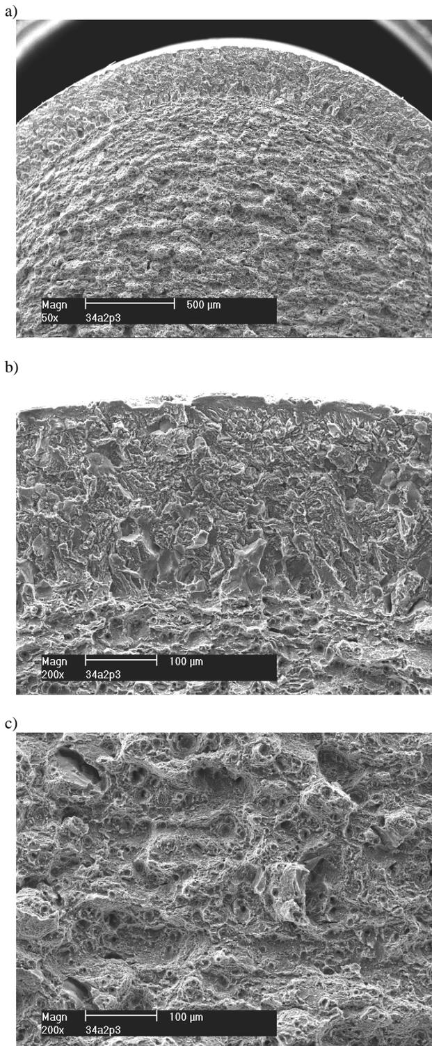
Fig. 14. SEM images of fracture surface of nitrided sample after SSRT tested in air: a) macroscopic view, b) modified layer, c) core of base metal
