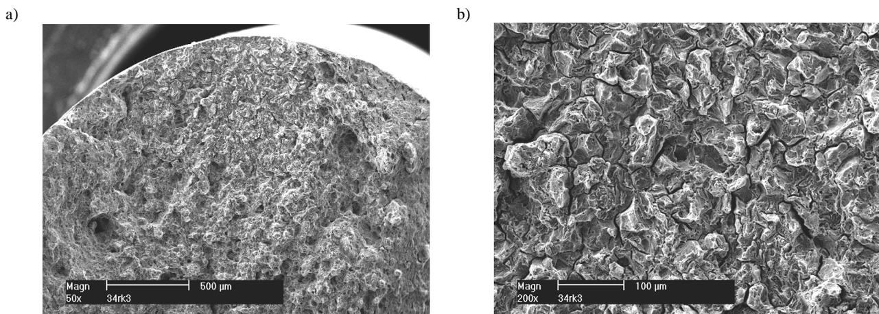
Fig. 13. SEM images of fracture surface of base metal sample after SSRT tested in acid solution under cathodic polarization: a) macroscopic view, b) core of base metal
