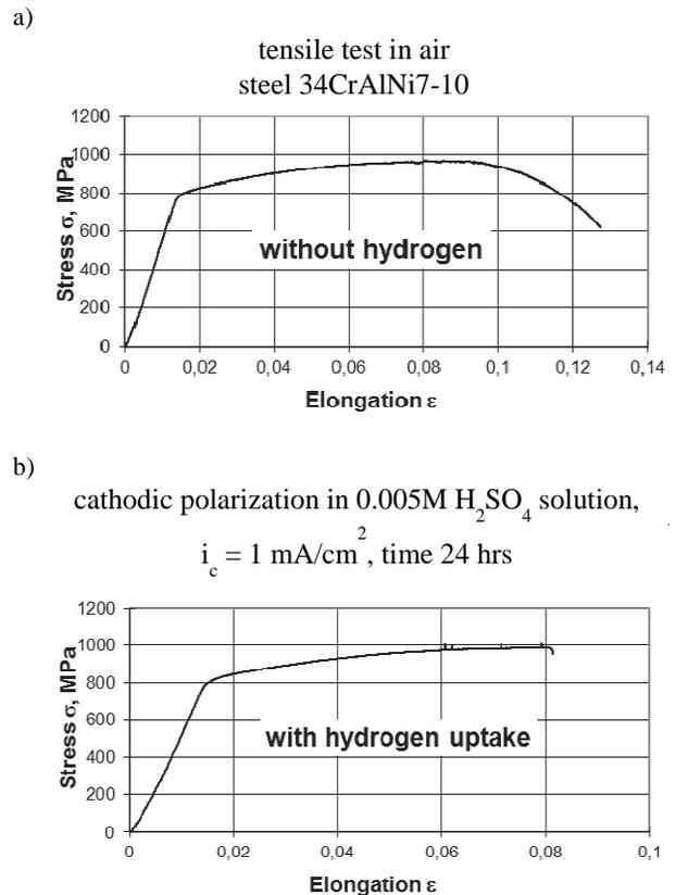
Fig. 1. Results of a tensile test for 34CrAlNi7-10 steel conducted: a) in air, b) in acid solution under cathodic polarization
