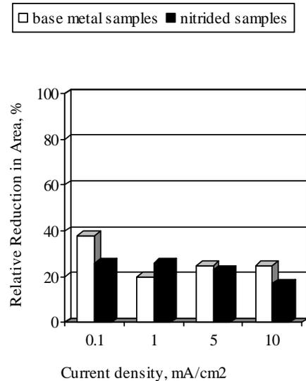
Fig. 10. Relative values of reduction in area vs. cathodic current density
