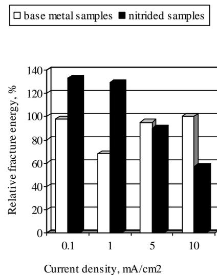
Fig. 11. Relative values of fracture energy vs. cathodic current density
