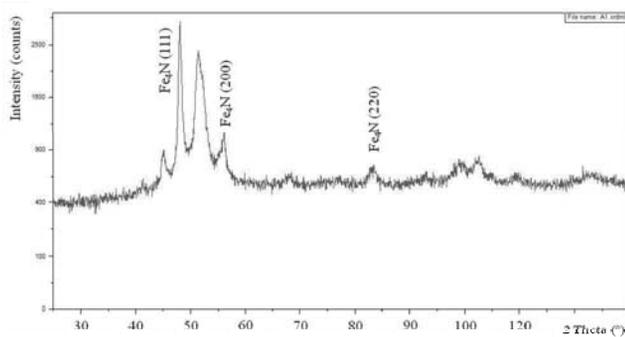
Fig. 6. The diffraction X-ray pattern for the compact nitride zone
