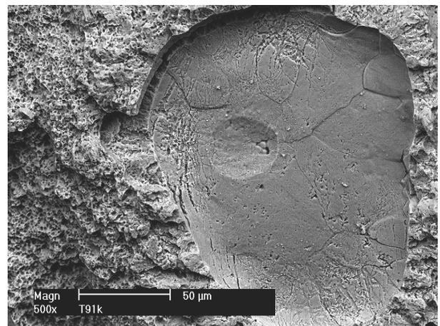
Fig. 2. The hydrogen blister in weld metal of HSLA steel S690Q
