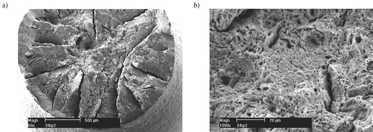
Fig. 12. SEM images of fracture surface of base metal sample after SSRT tested in air: a) macroscopic view, b) core of base metal
