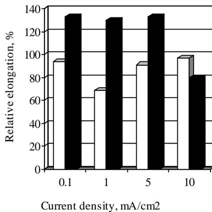
Fig. 9. Relative values of elongation vs. cathodic current density
