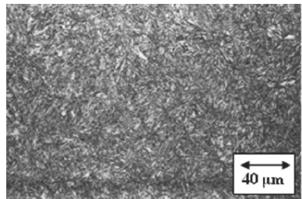
Fig. 4. Microstructure of 34CrAlNi7-10 steel. Nital etched. Light microscope
