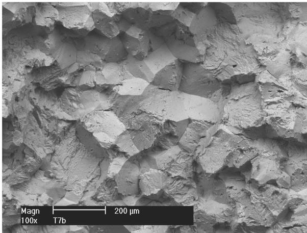
Fig. 3. Cold cracking in heat affected zone of HSLA steel S690Q
