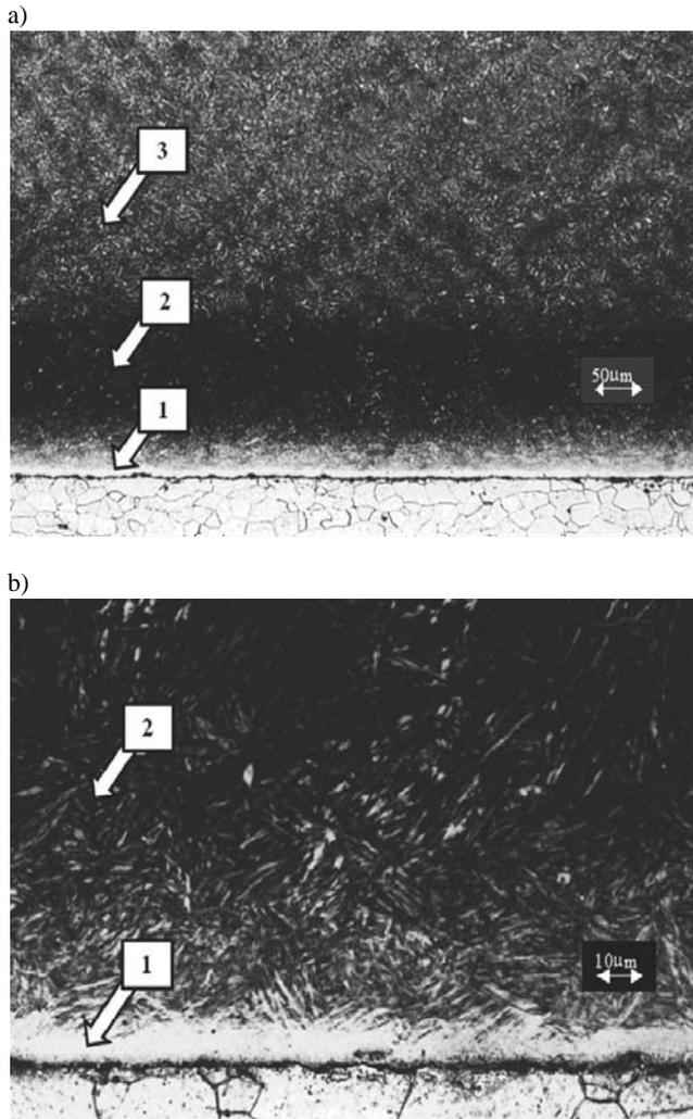
Fig. 5. Microstructure of the plasma nitrided surface layer on 34CrAlNi7-10 steel grade. Nital etched. Light microscope. a) 1-compound  $\gamma$  nitride zone, 2-diffusion zone, 3-tempered martensite (sorbite), b) a part of Fig. 1a; 1-compound  $\gamma$  nitride zone, 2-diffusion zone
