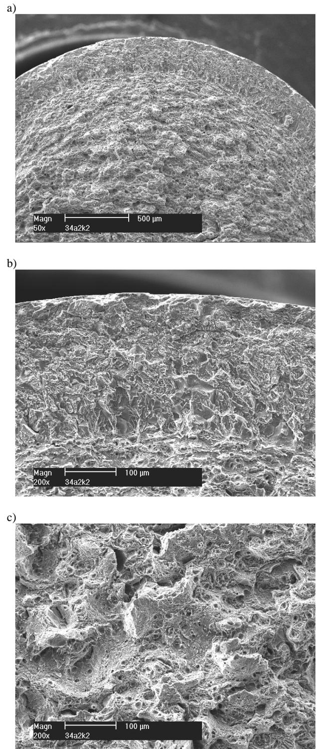
Fig. 15. SEM images of fracture surface of nitrided sample after SSRT tested in acid solution under cathodic polarization: a) macroscopic view, b) modified layer, c) core of base metal
