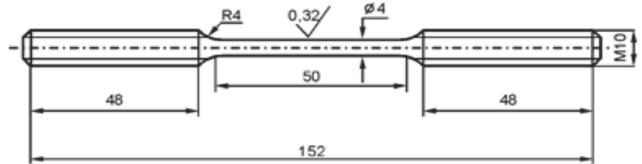
Fig. 7. The sample used for slow strain rate test
