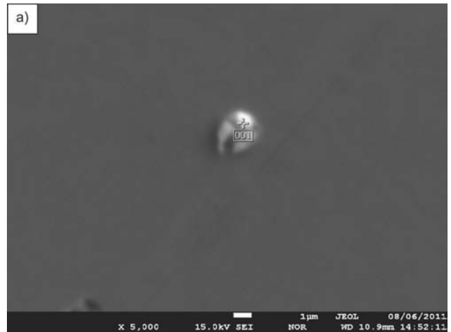
Fig. 6. Oxysulfide type non-metallic inclusion modified with rare earth elements; steel B after forging
