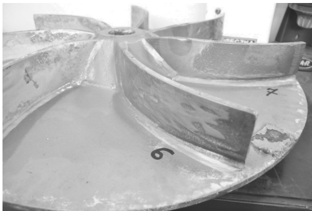
Fig. 22. Wear erosion of fan blade covered by the coating \text{NiCrBSi} (HVOF), \mu\text{HV} = 967
