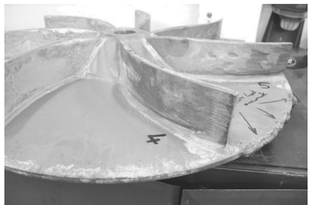
Fig. 20. Wear erosion of fun blade covered by the coating WC-Co-CrC-Ni (HVOF), \mu\text{HV} = 1195
