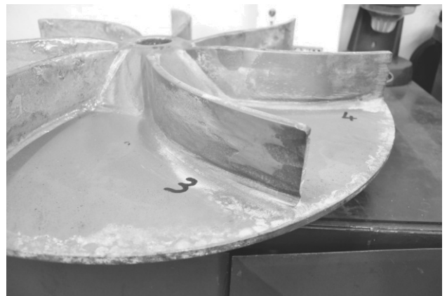
Fig. 19. Wear erosion of fun blade covered by the coating WC-Co +5%NiCrSiB (Plasma Spraying), \mu\text{HV} = 1218
