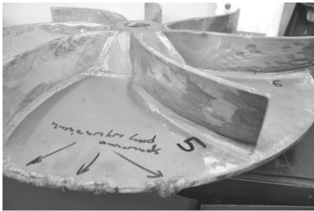
Fig. 21. Wear erosion of fan blade covered by the coating \text{Cr}_3\text{C}_2\text{-NiCr} (Plasma Spraying), \mu\text{HV} = 950
