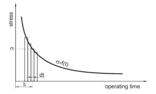
Fig. 12. Diagram of unsteady operating conditions of the object with continuous changes of stress
