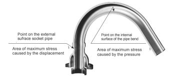
Fig. 8. Location of the points of maximum stresses in the pipeline
