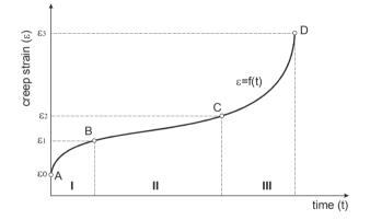
Fig. 2. The course of a typical creep curve. (I) – an unsteady process with a decreasing creep rate, (II) – a steady process with a constant creep rate, (III) – an unsteady process with an increasing creep rate
