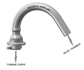
Fig. 1. General view of the research object: intermediate high-pressure pipeline
