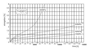
Fig. 3. Creep characteristics of the 14CrMoV6-3 steel [12]
