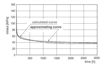
Fig. 9. Characteristics of stress redistribution on the outer surface of the bell
