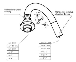
Fig. 4. Displacement values of pipeline connections in the cold and hot states
