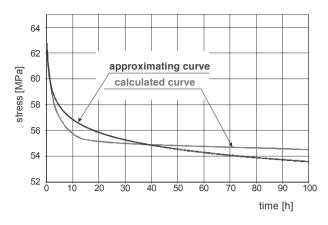
Fig. 10. Characteristics of stress redistribution in the point on the inner surface of the pipeline curve
