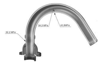
Fig. 7. Reduced stress distribution in the pipeline after the time of t=500 hours after the start-up of the power unit
