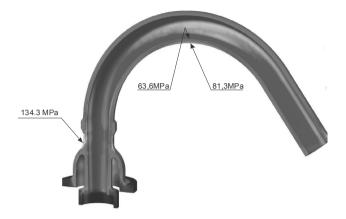
Fig. 5. Reduced stress distribution in the pipeline before start-up of the power unit
