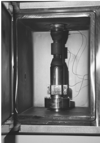
Fig. 4. Open chamber SPS apparatus with graphite die containing alumina powder before the sintering process
