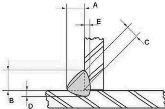
Fig. 3. Seam weld geometry
