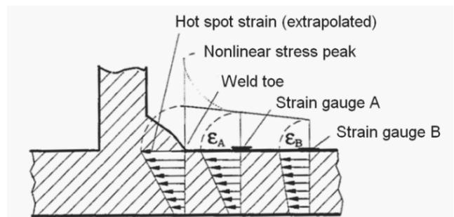
Fig. 1. Measurement of the hot spot strain range using the linear extrapolation method [15]
