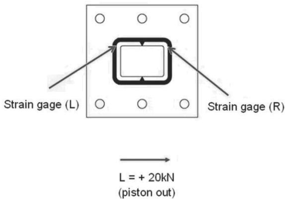
Fig. 5. Location of strain gages on the tube-to-plate sample
