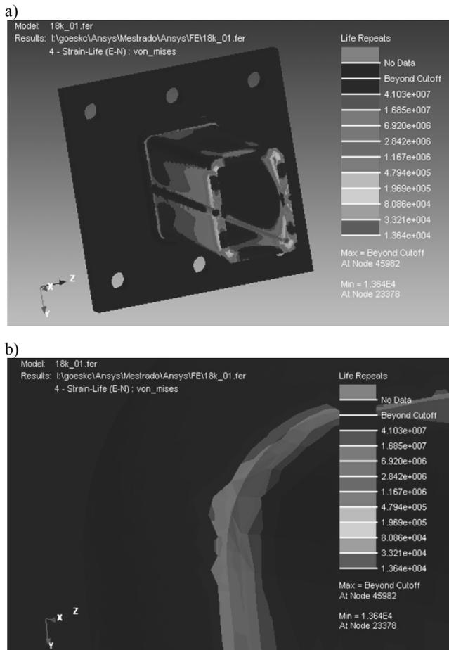
Fig. 9. Fatigue life distribution by FE-Fatigue (a) and detailed in the critical region (b)
