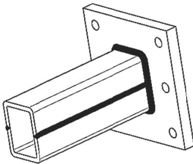
Fig. 2. Tube-to-plate sample
