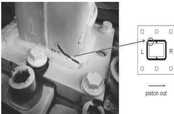
Fig. 10. Fatigue crack detection during the tests in laboratory
