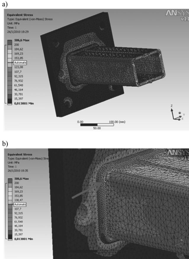
Fig. 8. Equivalent stress distribution predicted by FEA (a) and detailed in the critical region (b)
