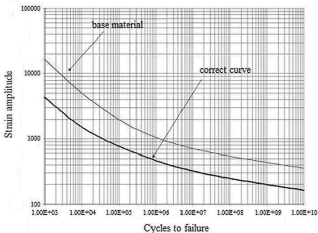
Fig. 6.  $\epsilon \times N$  curves obtained according to FAP7 database (base material) and fatigue test (correct curve)
