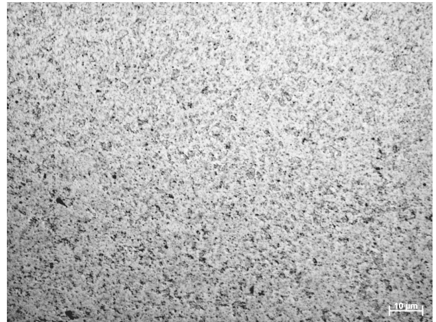
Fig. 6. Microstructure of extruded EN AW6061 with 5% addition of halloysite nanotubes after 24 h of milling
