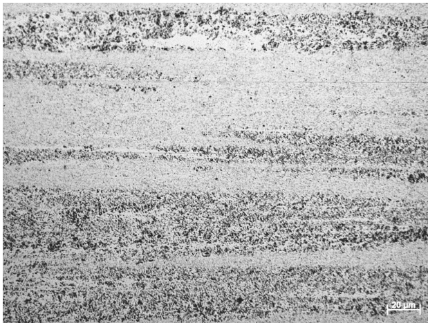
Fig 10. Microstructure of extruded EN AW6061 with 15% addition of halloysite nanotubes after 12 h of milling
