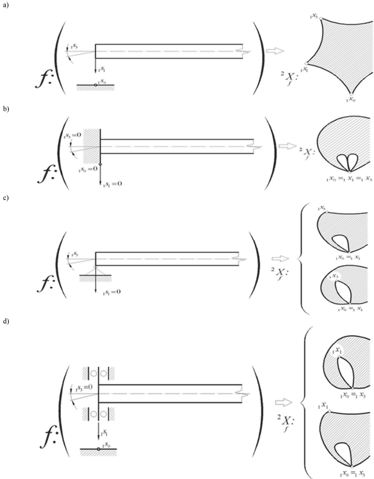
Fig. 1. Different boundary conditions of subsystems of beam system and their hypergraphs
