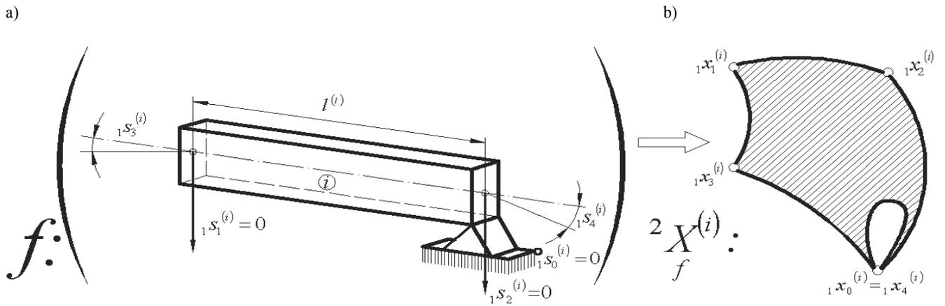
Fig. 2. Hypergraph (b) of model of flexibly vibrating beam (a) as graphical representation of transformations (3) and (4)
