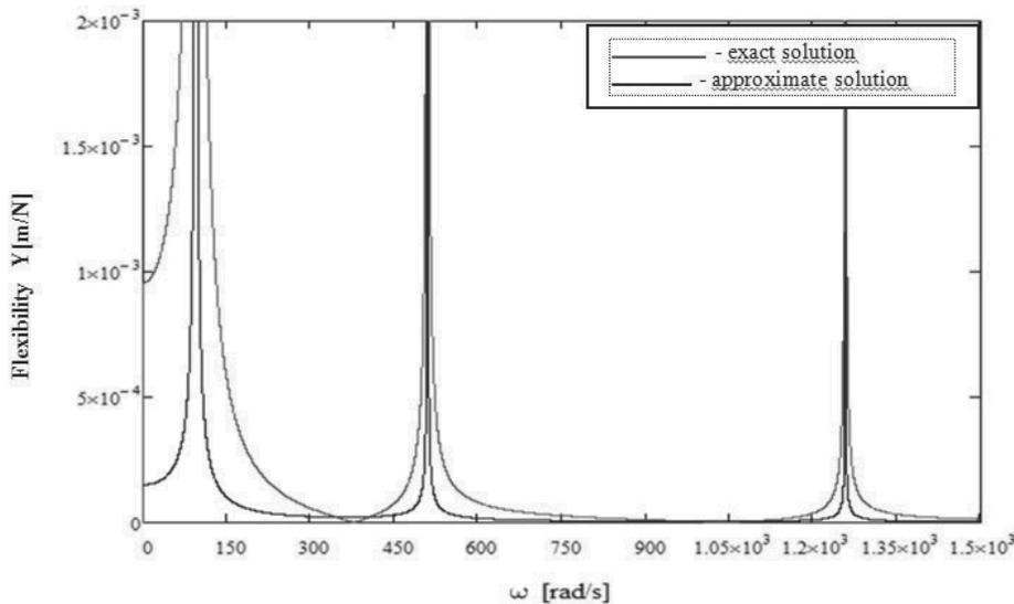
Fig. 6. The plot of absolute value of dynamical flexibility of the sum for  $n=1, 2, 3$  mode vibration for the system from Fig. 2a
