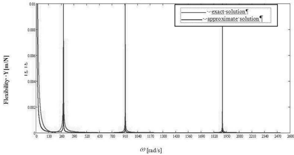
Fig. 7. The plot of absolute value of dynamical flexibility of the sum for  $n=1, 2, 3$  mode vibration for the system from Fig. 4a
