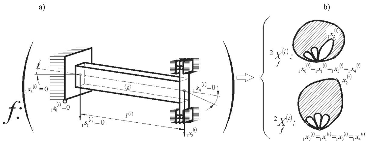
Fig. 4. Hypergraph (b) of model of flexibly vibrating beam (a) as graphical representation of transformations (3) and (4)
