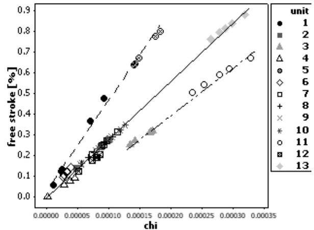
Fig. 9. Correlation plots relating the length of the free stroke to the value of  $\chi$  in simulations of shock absorber units
