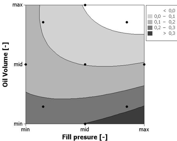
Fig. 8. Contour plot of the response surface of the free stroke length  $\mu$  vs. oil volume  $V_{oil}$  and the fill pressure  $p_{fill}$  obtained after 500 cycles
