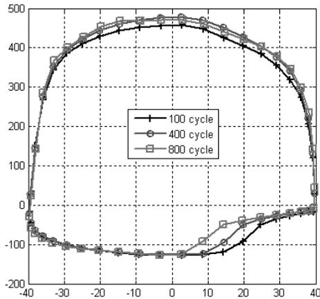
Fig. 6. The force-displacement characteristic of the transparent damper physical first test
