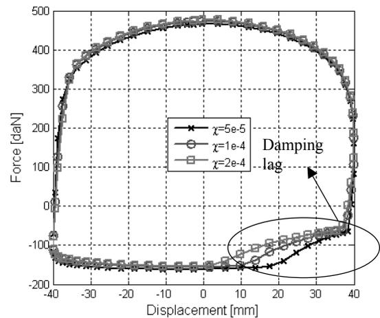
Fig. 5. The force-displacement characteristic of the transparent damper simulations
