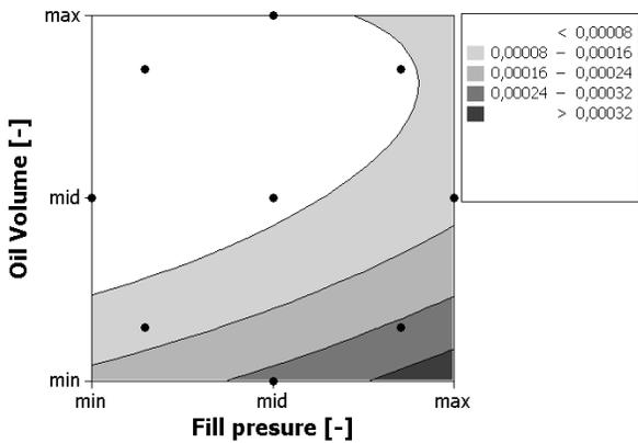
Fig. 7. Contour plot of the response surface of the parameter  $\chi$  vs. the oil volume  $V_{oil}$  and the fill pressure  $p_{fill}$  obtained after 500 cycles
