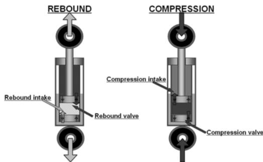
Fig. 1. Working principle of a double tube damper
