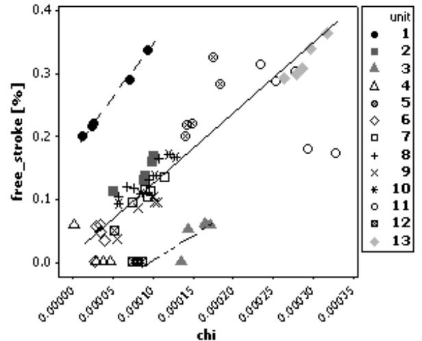
Fig. 10. Correlation plots relating the length of the free stroke to the value of  $\chi$  in experiments on shock absorber units
