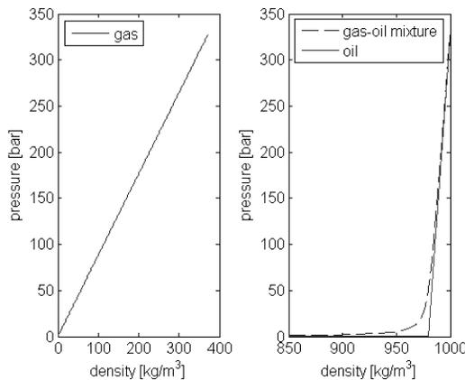
Fig. 2. Density-absolute pressure relation for gas and oil, and gas-oil mixture at constant temperature (ideal gas equation, isothermal fluid compressibility)
