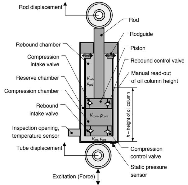
Fig. 3. Diagrammatic representation of transparent shock absorber
