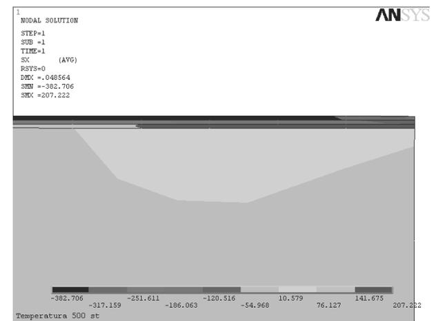
Fig. 9. Distribution of the simulated compression stresses in the gradient (Ti,Al)N coating deposited on to Al<sub>2</sub>O<sub>3</sub>+TiC type oxide tool ceramics substrate
