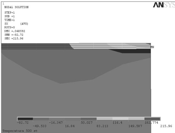
Fig. 14. Distribution of the simulated compression stresses in the single-layer Ti(C,N) coating deposited on to Al<sub>2</sub>O<sub>3</sub>+TiC type oxide tool ceramics substrate
