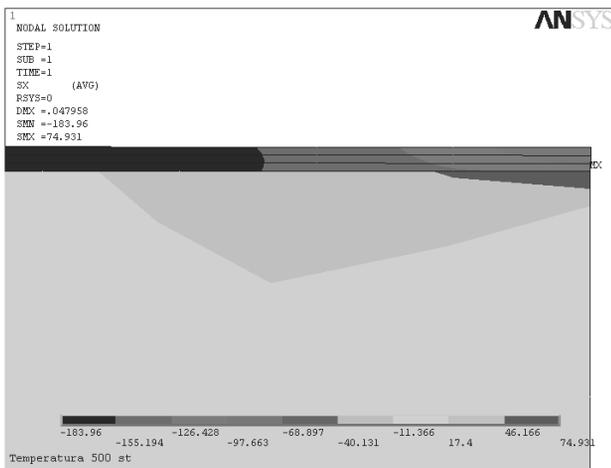
Fig. 4. Distribution of the simulated compression stresses in the single-layer (Ti,Al)N coating deposited on to cemented carbide substrate
