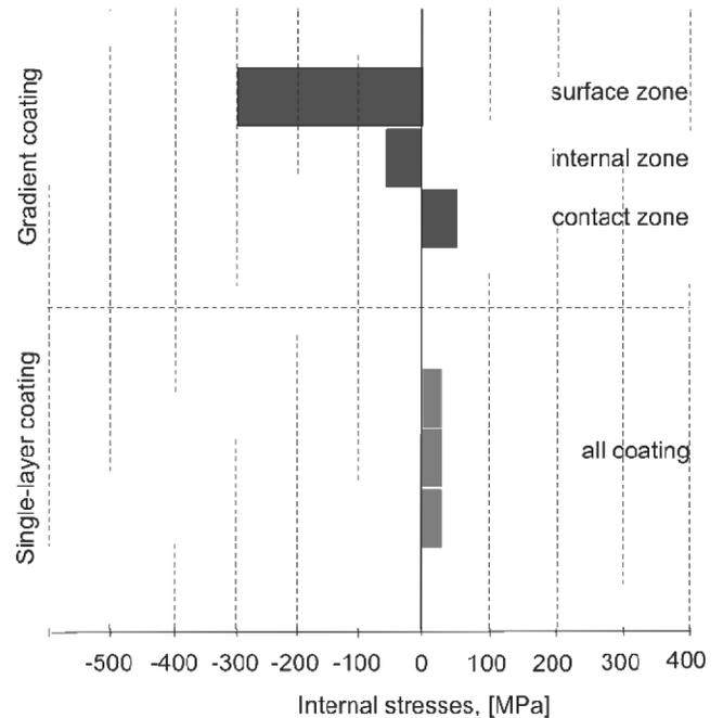
Fig. 20. Schematic distribution of stresses in the Ti(C,N) coatings deposited on cermet substrates obtained by computer simulation
