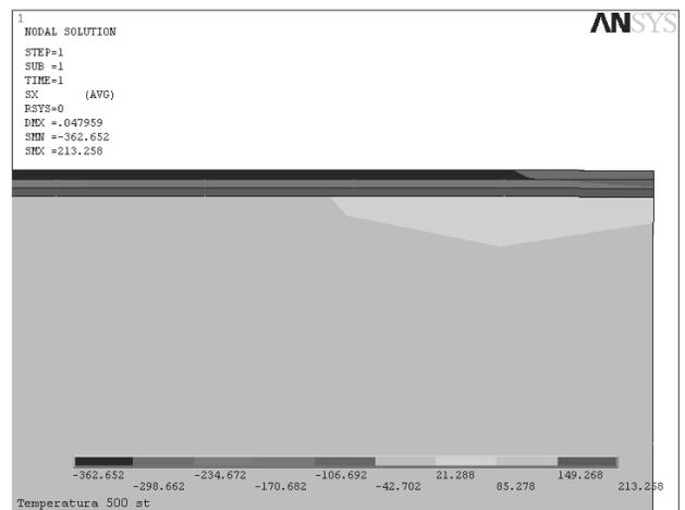
Fig. 5. Distribution of the simulated compression stresses in the gradient (Ti,Al)N coating deposited on to cemented carbide substrate
