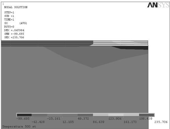
Fig. 10. Distribution of the simulated compression stresses in the single-layer Ti(C,N) coating deposited on to cemented carbide substrate
