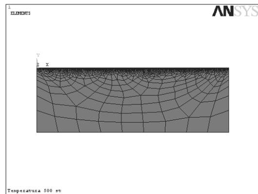
Fig. 1. True model subjected to discretization with deposited gradient and single-layer (Ti,Al)N and Ti(C,N) on different substrates
