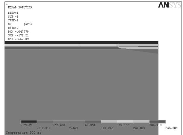
Fig. 11. Distribution of the simulated compression stresses in the gradient Ti(C,N) coating deposited on to cemented carbide substrate
