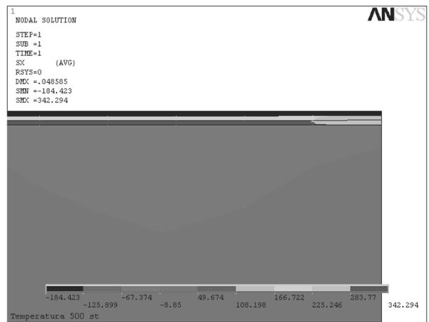
Fig. 15. Distribution of the simulated compression stresses in the gradient Ti(C,N) coating deposited on to Al<sub>2</sub>O<sub>3</sub>+TiC type oxide tool ceramics substrate
