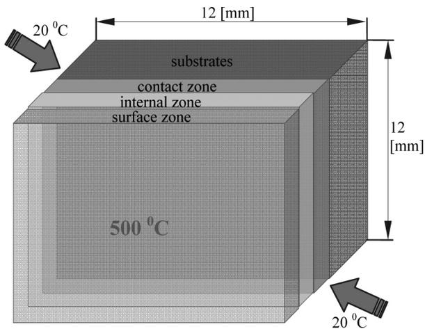
Fig. 2. Real model of gradient coatings
