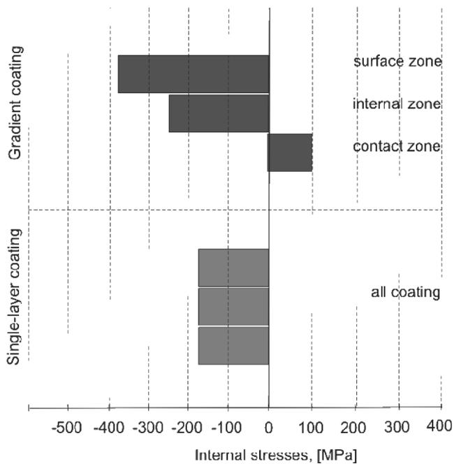
Fig. 18. Schematic distribution of stresses in the (Ti,Al)N coatings deposited on Al<sub>2</sub>O<sub>3</sub>+TiC type oxide tool ceramics substrate obtained by computer simulation
