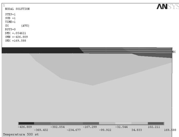
Fig. 6. Distribution of the simulated compression stresses in the single-layer (Ti,Al)N coating deposited on to cermet substrate
