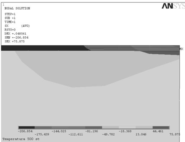
Fig. 8. Distribution of the simulated compression stresses in the single-layer (Ti,Al)N coating deposited on to Al<sub>2</sub>O<sub>3</sub>+TiC type oxide tool ceramics substrate
