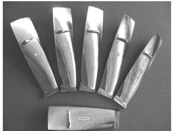
Fig. 1. Blades of zero compression stage of Russian aircraft engine turbine made of titanium alloy WT3-1, Tables 1 and 2
