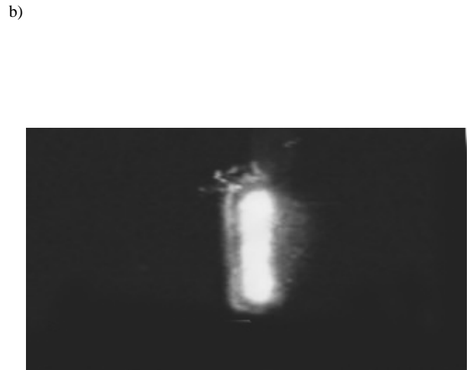
Fig. 9. A view of powder laser HPDL hardfacing process with side powder feeding system (a) and thermovision image of the laser beam focused on the surface of the titanium alloy plate to be hardfaced (b)
