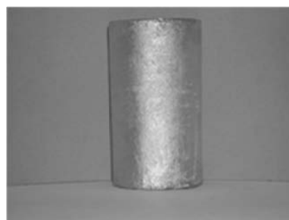
Fig. 29. The silumin coat on the cast iron linear bushing dipped into the bath AlSi9Cu1,5Ni1,5Mg0,5 in the industrial conditions.
