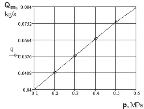
Fig. 8. The relationship between the blasting machine productivity  $Q_m$  and pressure  $p$  in the hopper of wet abrasive peening cyclic system
