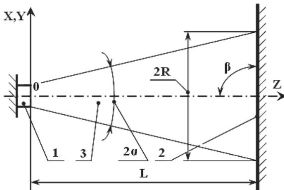
Fig. 2. Scheme of the blast that run out from the nozzle with circular cross-section: 1 - nozzle; 2 - surface; 3 - blast;  $2\alpha$  - cone angle;  $\beta$  - impinging angle;  $R$  - the blast trace radius on treated surface;  $L$  - the perpendicular length between treated surface and the end of the nozzle
