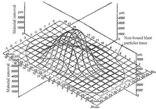
Fig. 5. a) material removal after abrasive blasting: compresses air pressure  $p = 0.5$  MPa, processing time - 120 s, grid size - 60, the ratio of solid components in blast to liquid components - 1 : 4, impinging angle -  $45^\circ$ ; b) trace shape and topography after treating flat unmoved surface with the stationary blast apparatus
