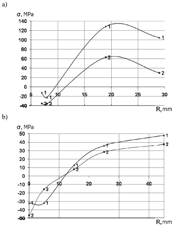
Fig. 23. Distribution diagram of residual stresses along the jet track on the treated surface: 1 - residual stresses  $\sigma_{xx}$ ; 2 - residual stresses  $\sigma_{yy}$ ; a) processing time - 10 min; b) processing time - 20 min
