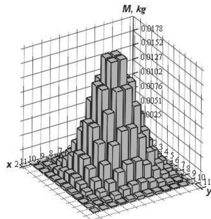
Fig. 10. The mass distribution after non-bound blast particles treatment
