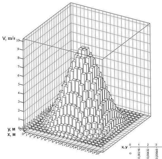
Fig. 16. Blast velocity distribution in a cross-section:  $d_s = 0.01$  m;  $L = 0,1$  m;  $\Delta p = 0,5 \times 10^5$  Pa;  $\alpha = \pi/18$ ;  $\rho_c = 1280$  kg·m<sup>-3</sup>;  $a = 0.14$ ;  $k_1 = 1.5$ ;  $k_2 = 2$ ;  $\xi = 1$
