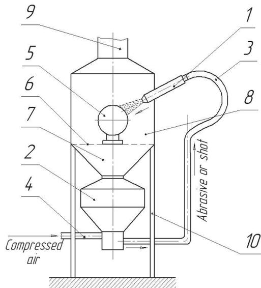
Fig. 26. Shot-peening system equipped by shot hopper: 1 - nozzle; 2 - hopper; 3 - hose; 4 - pipe for supplying compressed air; 5 - machine part; 6 - table; 7 - conical bunker; 8 - working chamber; 9 - incoming pipe cyclone; 10 - holders
