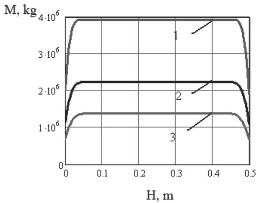
Fig. 18. Mass distribution along the treated surface trajectory for various distances between surface being treated and the nozzle 1 -  $L = 0.4$  m; 2 -  $L = 0.5$  m; 3 -  $L = 0.6$  m
