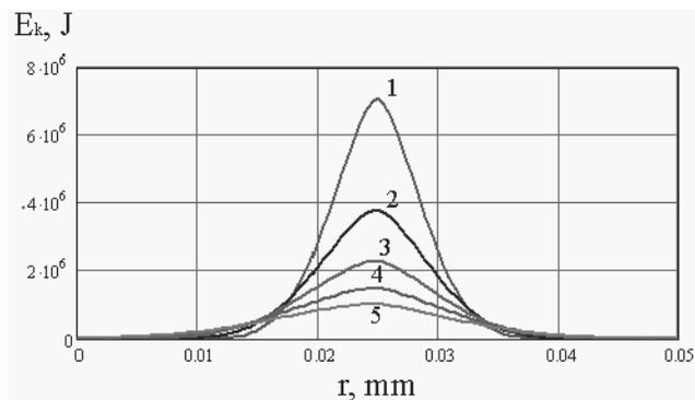
Fig. 20. Kinetic energy distribution along the radius of the rotary plate from perpendicular distance between surface being treated and the nozzle end for the eccentricity  $x_c = 25$  mm:
