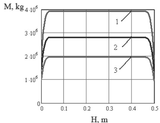
Fig. 17. Mass distribution along the treated surface trajectory for various velocities of its movement: 1 -  $V = 0.005$  mps; 2 -  $V = 0.007$  mps; 3 -  $V = 0.01$  mps
