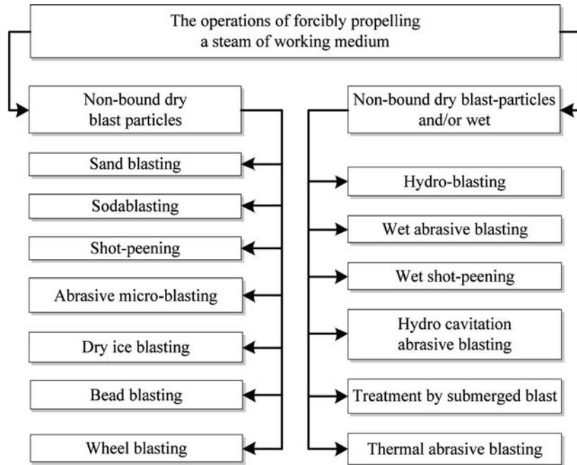
Fig. 3. The operations of forcibly propelling a steam of working medium
