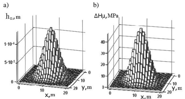
Fig. 21. Distribution diagram of quality characteristics on the surface after non-bound blast particles treatment: a) depth of hardening layer  $h_n$ , b) change of microhardness  $\Delta H\mu$
