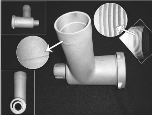
Fig. 1. Components treated by the blast of angular abrasive
