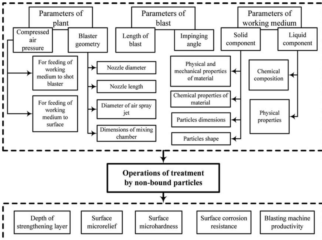
Fig. 4. Parameters of treatment by non-bound blast particles, and quality characteristics of the machine parts surfaces
