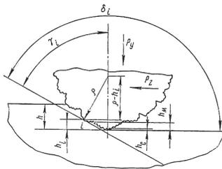
Fig. 6. Scheme of interaction between the non-bound particle and the surface
