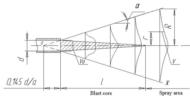
Fig. 11. Blast that flows for the round cross-section nozzle
