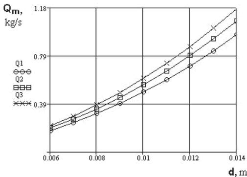
Fig. 7. The relationship between the blasting machine productivity  $Q_m$  and the nozzle diameter  $d_s$ :  $Q_1$  - for  $\Delta p = 0,04 \text{ MPa}$ ;  $Q_2$  - for  $\Delta p = 0,05 \text{ MPa}$ ;  $Q_3$  - for  $\Delta p = 0,06 \text{ MPa}$
