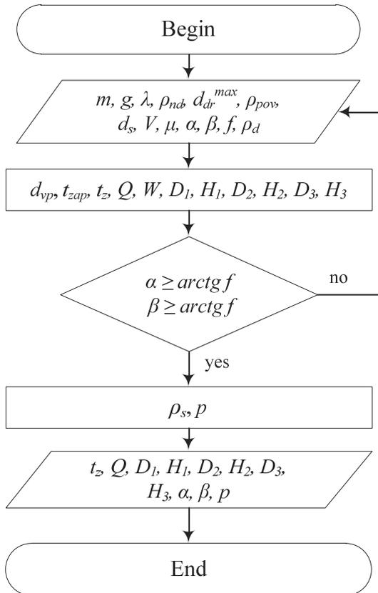
Fig. 28. Algorithm of shot hopper calculations
