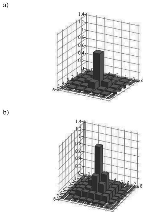
Fig. 25. The material layer thickness removed by wet abrasive jet from flat specimen distribution: a) processing time - 10 min; b) processing time - 20 min
