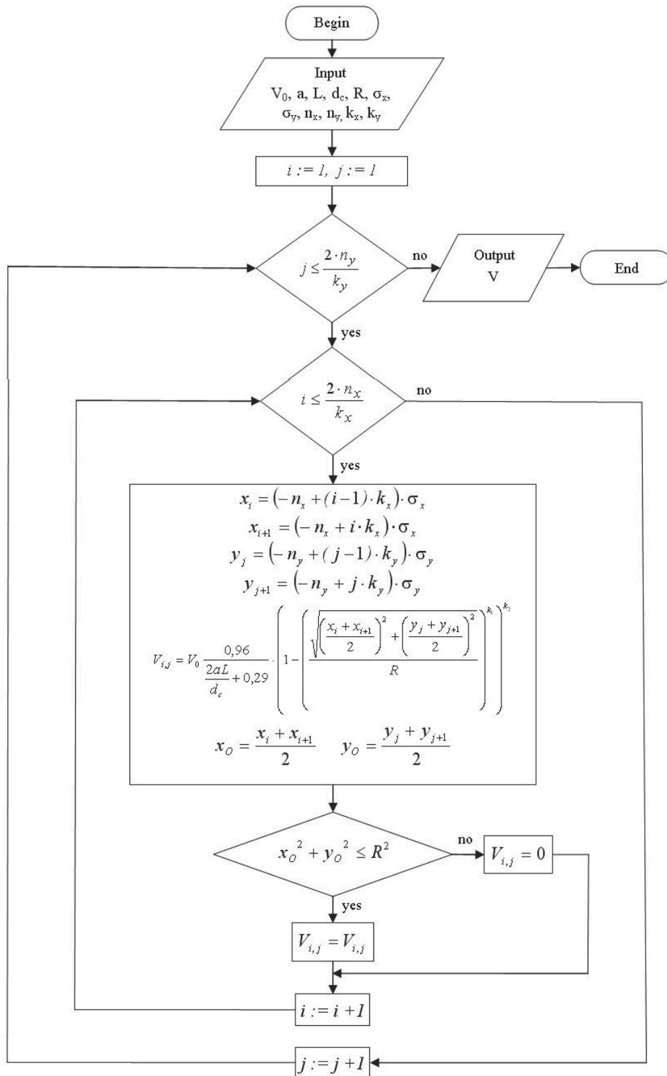
Fig. 15. Flowchart for blast velocity distribution calculations  $V_{ij}$
