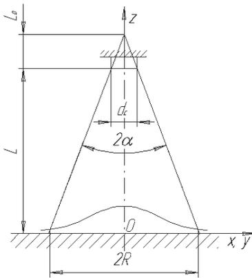
Fig. 9. Scheme for determining standard deviation for mass working medium distribution
