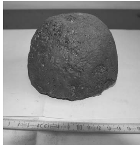
Fig. 33. Small "craters" on the surface of the investigated element
