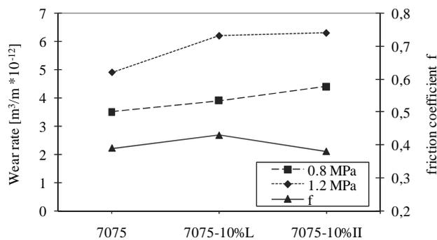
Fig. 6. Wear rate and friction coefficient and of the matrix 7075 and composite reinforced with 10% vol.  $\text{Al}_2\text{O}_3$  after T6 examined under pressures of 0.8 and 1.2 MPa
