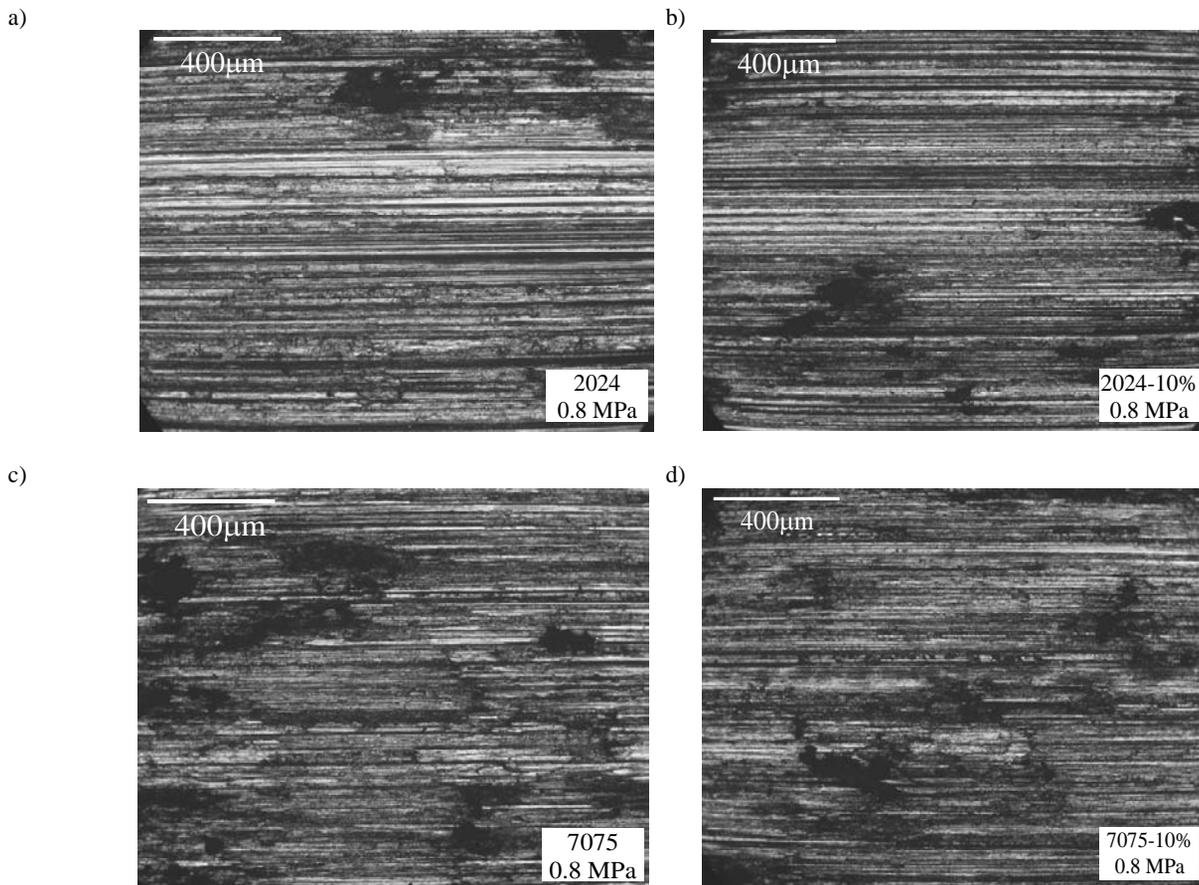
Fig. 7. The worn surfaces of specimens tested under pressure of 0.8 MPa. Unreinforced 2024 alloy (a) and unreinforced 7075 alloy (c), 2024 alloy based composite material reinforced with 10 vol. % of  $\text{Al}_2\text{O}_3$  Saffil fibres (b), and 7075 based composite material reinforced with 10% of  $\text{Al}_2\text{O}_3$  Saffil fibres (d)
