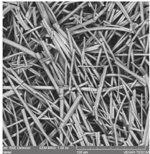
Fig. 1. Preform produced from the blended Saffil  $\text{Al}_2\text{O}_3$  and graphite fibres
