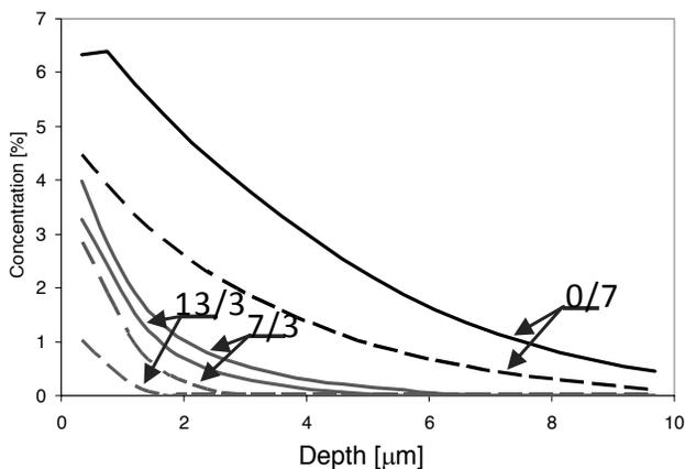
Fig. 11. Depth profiling showing Al concentration in counterparts surface after wear test against composite containing 7% of  $\text{Al}_2\text{O}_3$  fibres (0/7), reinforced with 7% of  $\text{Al}_2\text{O}_3$  and 3% of graphite (7/3), and reinforced with 13% of  $\text{Al}_2\text{O}_3$  and 3% of graphite (13/3). Continuous line represents maximum, broken line minimum concentration of Al
