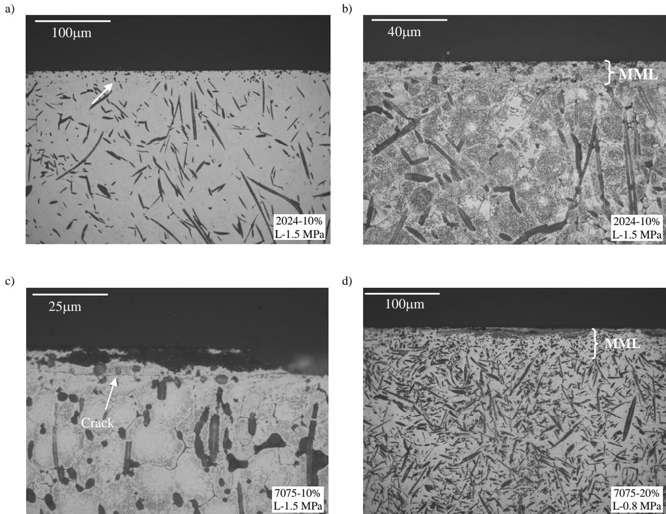
Fig. 10. Deformation in subsurfaces of 2024 and 7075 alloys based composite materials with Saffil fibres created under various loads
