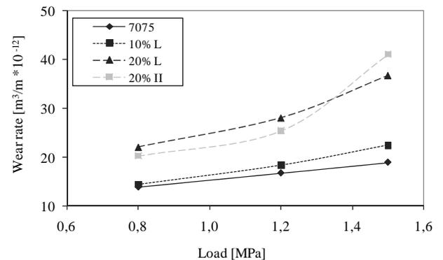
Fig. 3. Effect of load and orientation of Saffil  $\text{Al}_2\text{O}_3$  fibres on wear of 7075 unreinforced matrix and composite materials with 10% and 20 vol. % of  $\text{Al}_2\text{O}_3$  fibres
