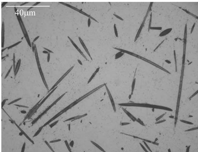
Fig. 2. Microstructure of the composite 7075+10 vol. %  $\text{Al}_2\text{O}_3$  in surface with planar random orientation of fibres
