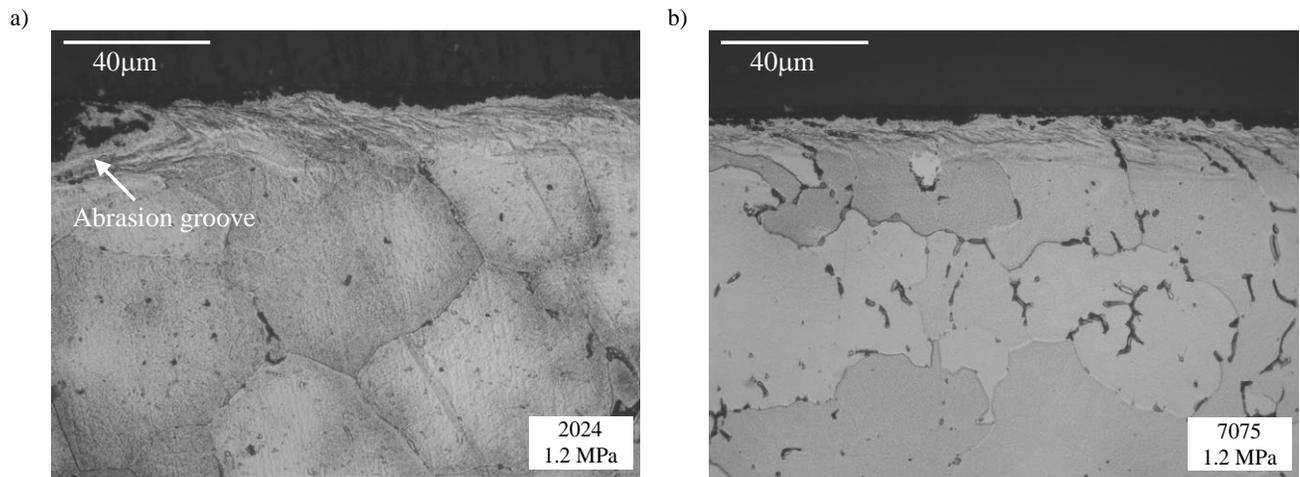
Fig. 9. Longitudinal cross-section of subsurfaces of unreinforced specimens of 2024 and 7075 alloys after T6 worn under pressure of 1.2 MPa
