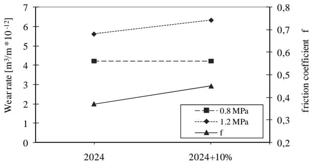
Fig. 5. Wear rate and friction coefficient of the unreinforced matrix 2024 and 2024 Al based composite material reinforced with 10 vol.%  $\text{Al}_2\text{O}_3$  Saffil fibres after T6 examined under pressures of 0.8 and 1.2 MPa
