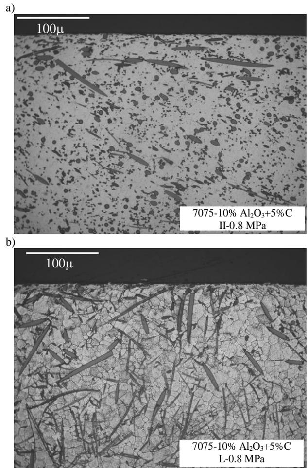
Fig. 12. Wear surface of 7075+10 vol. %  $\text{Al}_2\text{O}_3$ +5%C specimen with normal (a) and planar random orientation of fibres to friction surface (b) after test performed under pressure of 0.8 MPa
