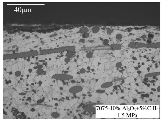
Fig. 13. Wear surface of 7075+10%  $\text{Al}_2\text{O}_3$  Saffil+5%C specimen with planar random orientation of fibres to friction surface
