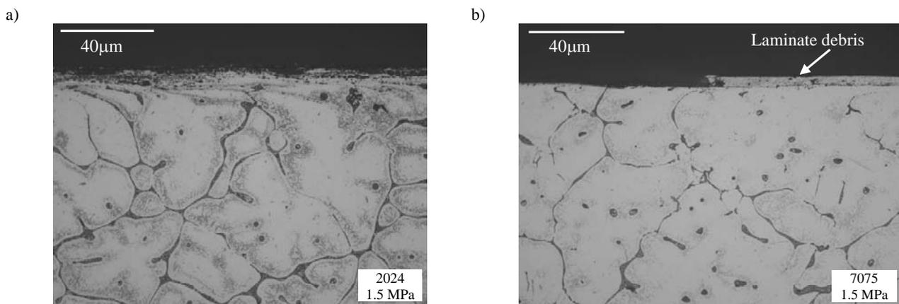
Fig. 8. Longitudinal cross-section of subsurfaces of unreinforced specimens of 2024 and 7075 worn under pressure of 1.5 MPa. Slightly deformed crystals with rubbed debris in 2024 specimen (a), compact delamination of 7075 specimen (b)
