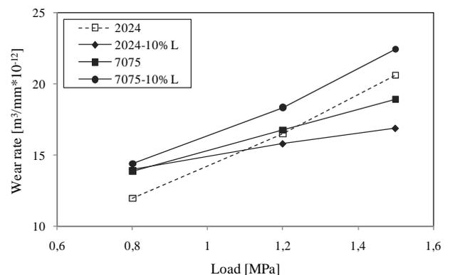
Fig. 4. Effect of load and orientation of  $\text{Al}_2\text{O}_3$  Saffil fibres on wear of 2024 and 7075 matrix alloys and composite materials on their bases
