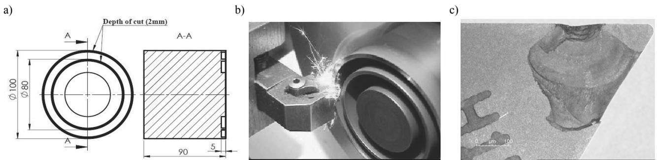
Fig. 2. a) Specimen form, (b) orthogonal cutting, and (c) the carbides in the matrix of the materials create grooves by wear on the tool
