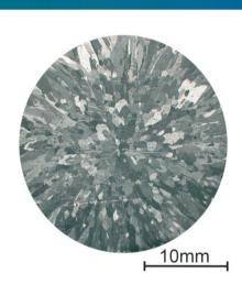
The research paper made by S T. Wróbel and J. Szajnar on "The influence of inoculants sort on pure Al structure" on a page 92 analyses the problem concerning inoculation of pure aluminum primary
