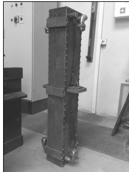
Fig. 1. Copper crystalliser cooled with water, simulating the process of continuous casting of steel
