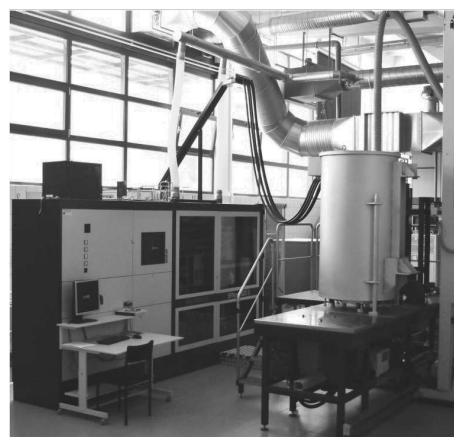
Fig. 1. IonBond BPXPRO325S apparatus for CVD aluminizing
