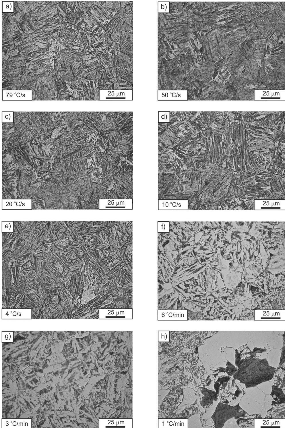
Fig. 6. Structures obtained after cooling the specimens from the deformation temperature of 1100°C with a rate: a) 79°C/s, b) 50°C/s, c) 20°C/s, d) 10°C/s, e) 4°C/s, f) 6°C/min, g) 3°C/min, h) 1°C/min
