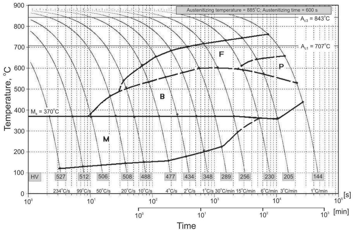
Fig. 1. Diagram of supercooled austenite transformations of investigated steel
