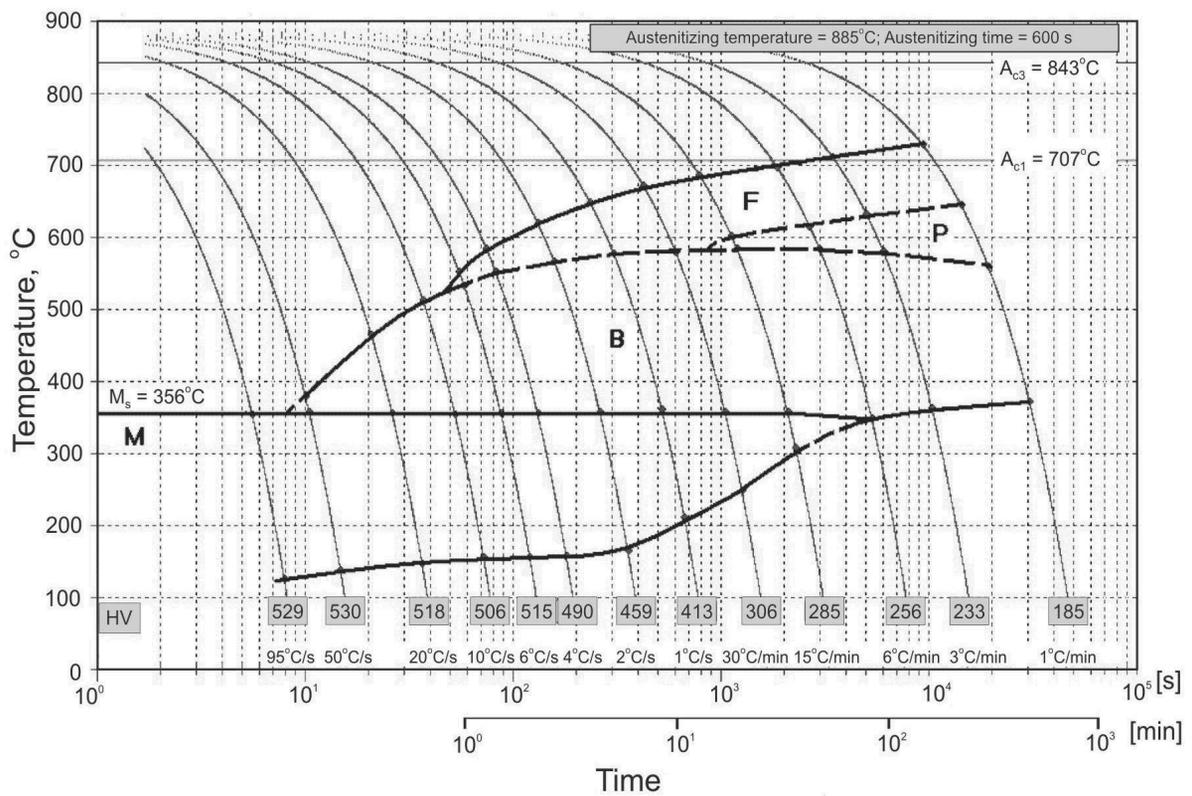
Fig. 3. Diagram of supercooled plastically-deformed austenite transformations of investigated steel; deformation temperature: 885°C
