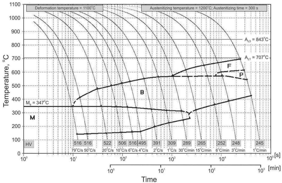
Fig. 5. Diagram of supercooled plastically-deformed austenite transformations of investigated steel; deformation temperature: 1100°C
