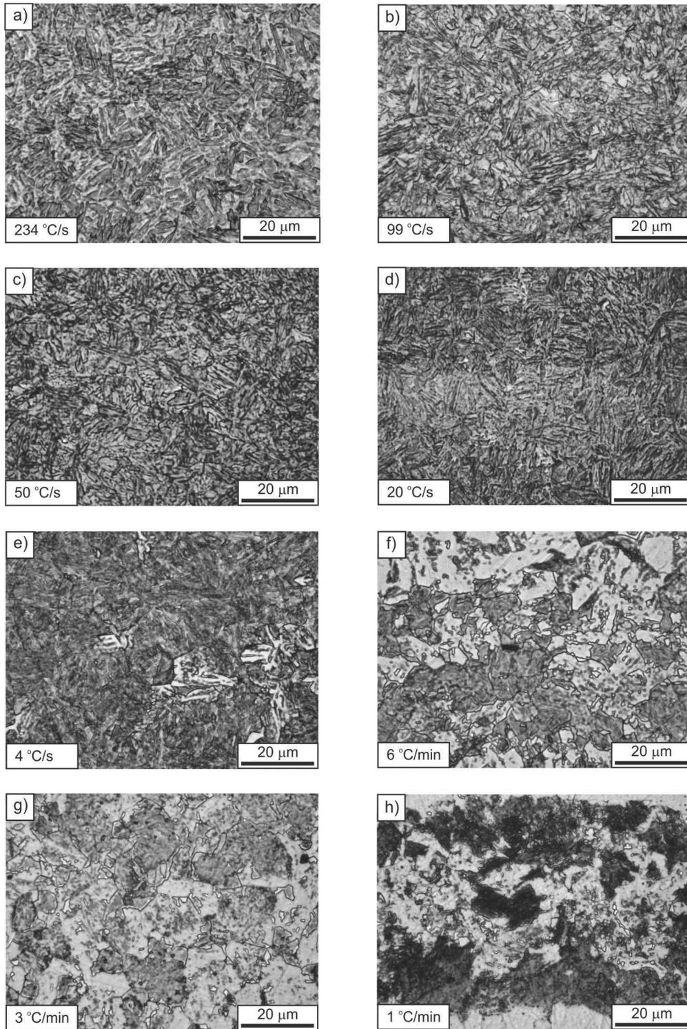
Fig. 2. Structures obtained after cooling the specimens from the austenitizing temperature of 885°C with a rate: a) 234°C/s, b) 99°C/s, c) 50°C/s, d) 20°C/s, e) 4°C/s, f) 6°C/min, g) 3°C/min, h) 1°C/min
