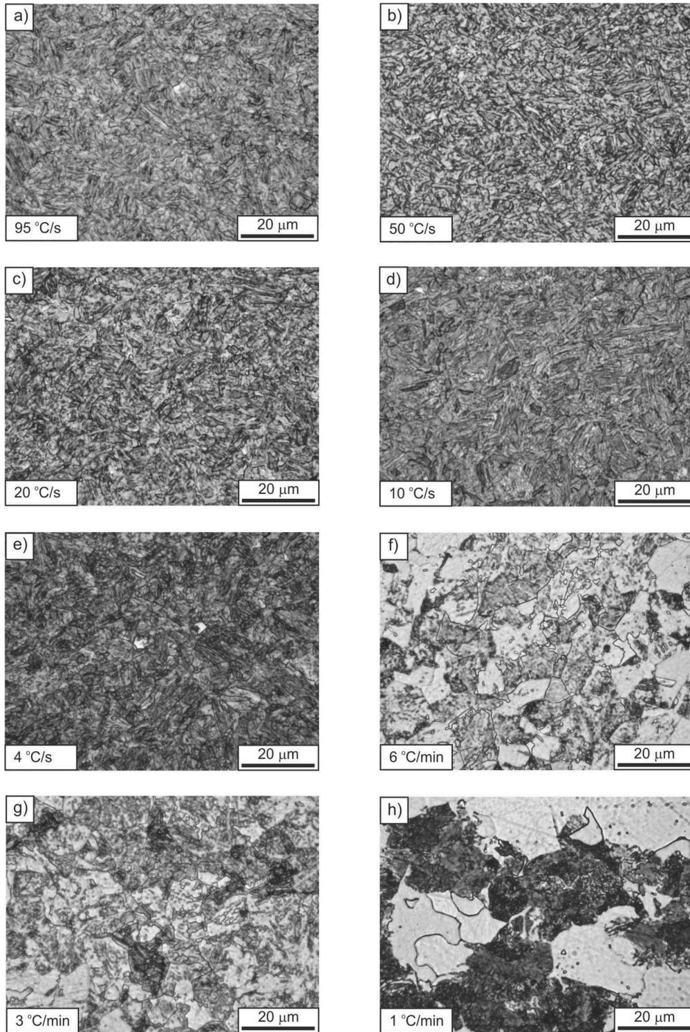
Fig. 4. Structures obtained after cooling the specimens from the deformation temperature of 885°C with a rate: a) 95°C/s, b) 50°C/s, c) 20°C/s, d) 10°C/s, e) 4°C/s, f) 6°C/min, g) 3°C/min, h) 1°C/min
