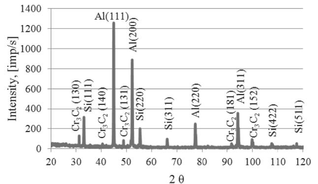
Fig. 8. The result of X-ray phase analysis of the AlSi11/CrFe30C8 composite castings
