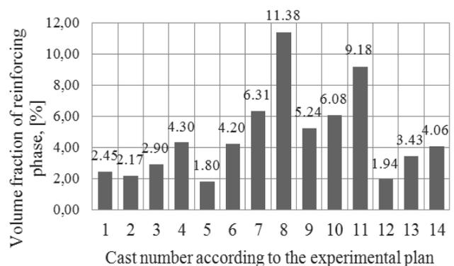
Fig. 4. Areal fraction of reinforcement phase in obtained composite castings
