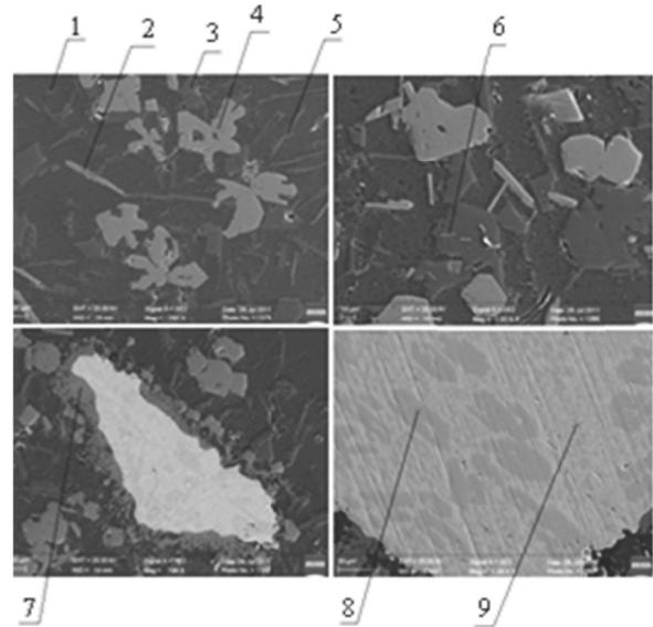
Fig. 7. Example of microstructures obtained AlSi11/CrFe30C8 composites with CrFe30C8 particles size 200 μm with specified characteristic points to the analysis
