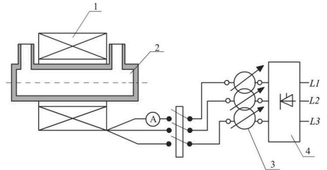
Fig. 1. Experimental stand for production of composites under electromagnetic field: 1 - inductor, 2 - shell mould, 3 - autotransformer, 4 - inverter
