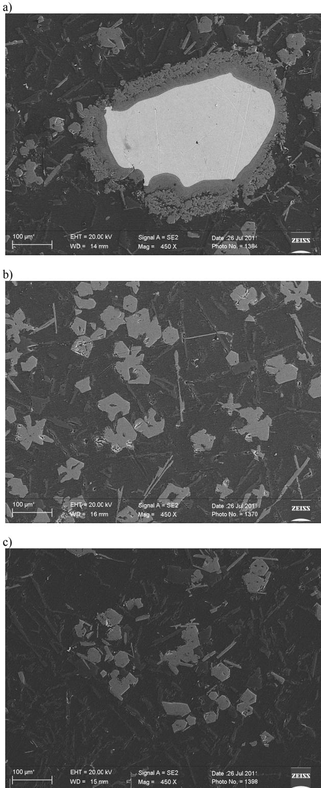
Fig. 6. Example of microstructure of AlSi11/CrFe30C8 composite samples with particles size of 200 [μm] for different frequency: a) 50 [Hz], b) 75 [Hz], c) 100 [Hz]
