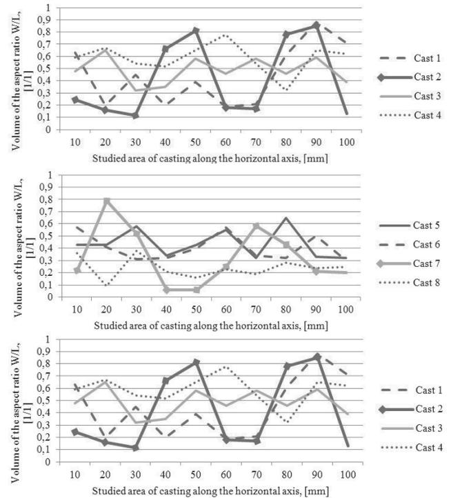
Fig. 5. The average value of the aspect ratio along the horizontal axis in AlSi11/CrFe30C8 composite castings produced under electromagnetic field
