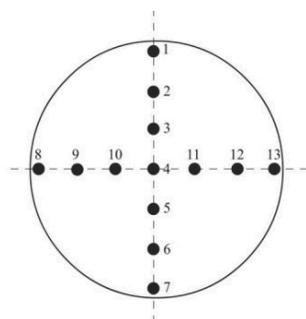
Fig. 3. Measurement points on composite samples
