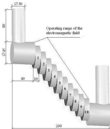
Fig. 2. Preparation method of samples for metallographic testing
