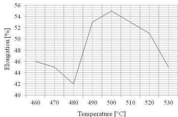
Fig. 7. Elongation vs. homogenization temperature
