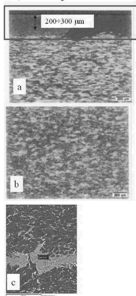
Fig. 2. OM microstructures: a) on the surface layer, b) in the core of the sample and c) SEM microstructure showing the presence of microsegregation
