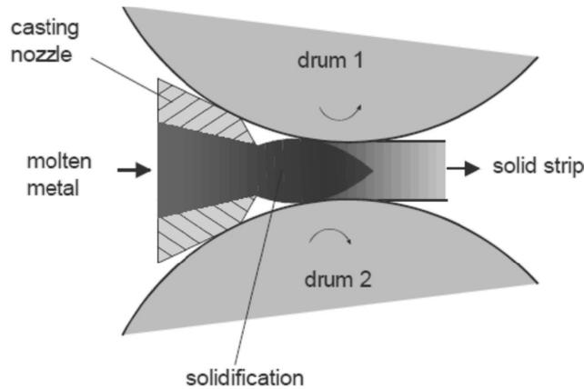
Fig. 1. Schematic representation of the continuous casting process
