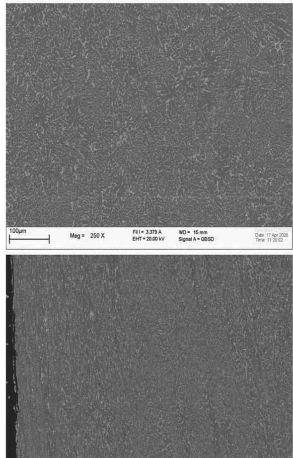
Fig. 6. Distribution of the intermetallic compounds in the core and on the surface layer of the homogenized alloy with the relative SEM microstructures
