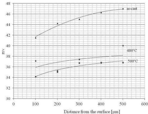
Fig. 8. Vickers hardness evolution in the homogenized and as cast samples
