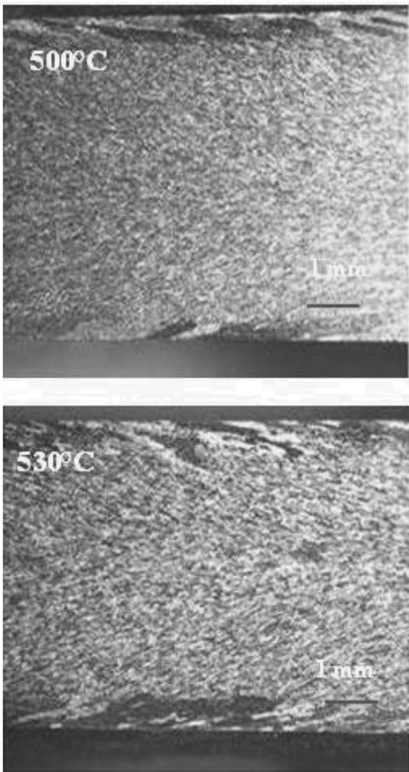
Fig. 5. Evolution of the grain structures across the cross-section of the samples annealed at 500°C and 530°C
