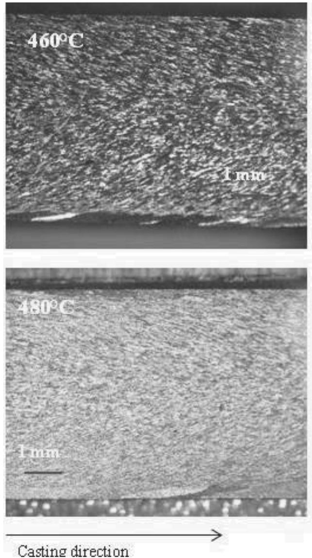
Fig. 4. Evolution of the grain structures across the cross-section of the samples annealed at 460°C and 480°C
