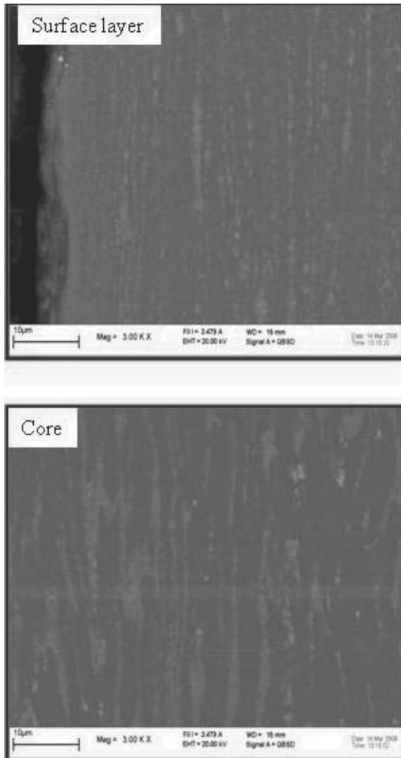
Fig. 3. SEM microstructure showing the evolution of the grain structures on the surface layer (top) and in the core (bottom) of the samples
