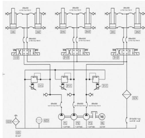
Fig. 8. The corresponding circuit hydraulic scheme
