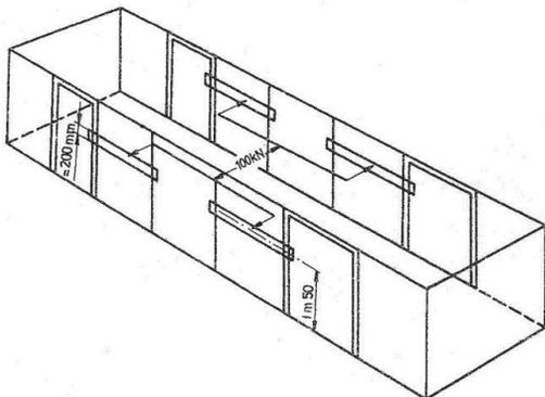
Fig. 1. The strength test of the side walls of the wagon [3]
