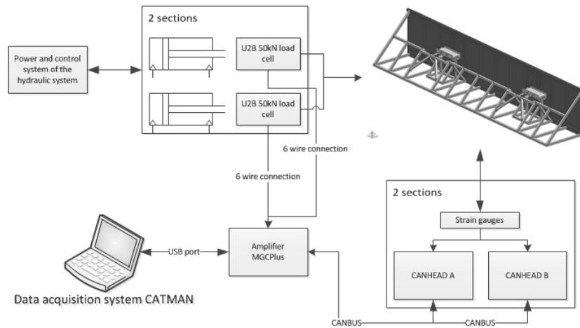
Fig. 9. The measuring circuit
