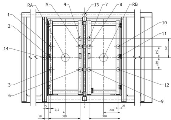
Fig. 15. The distribution and numbering of strain gauges
