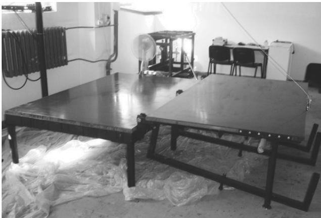
Fig. 10. The manufacturing stand for the manufacture of composite panels
