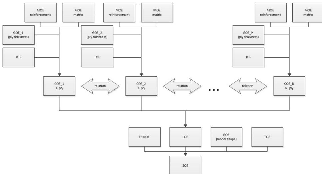
Fig. 4. The structure of the feature-based method
