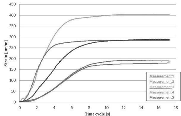
Fig. 16. Comparison of results of deformation measurements of 1-5, rosette B1
