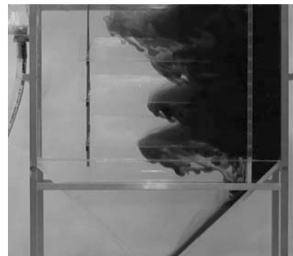
Fig. 24. Visualization of cross-current flow for q=0.5 m/h
