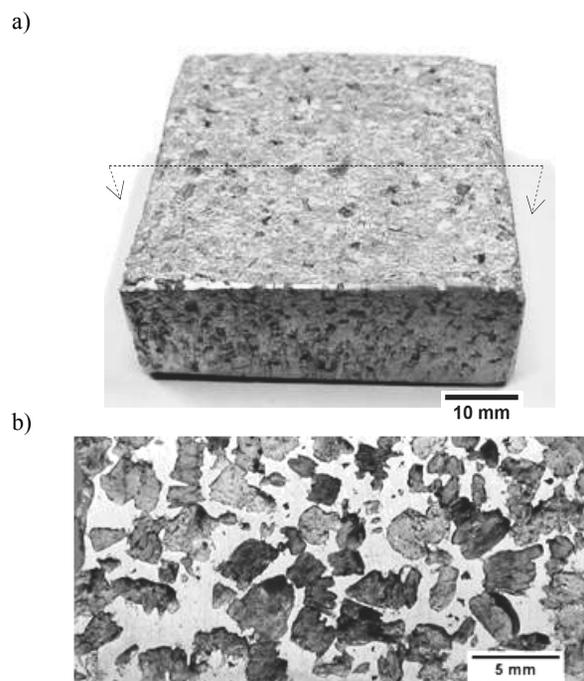
Fig. 5. Typical sample produced by thixoinfiltration of AA7075 into a layer of fine vermiculite particles; (a) general aspect; (b) transversal section
