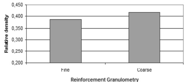
Fig. 9. Relative density of the AA7075/SiO<sub>2</sub>-MgO-Al<sub>2</sub>O<sub>3</sub> composite produced
