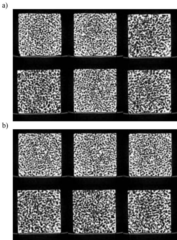
Fig. 6. X-ray tomography images of parallel planes of typical samples of AA7075 matrix MMC, produced by thixoinfiltration into (a) fine, (b) coarse reinforcing vermiculite particles
