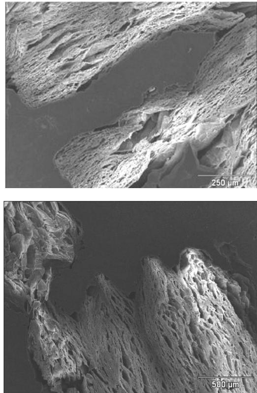
Fig. 7. SEM images of a section of a typical AA7075/ $\text{SiO}_2\text{-MgO-Al}_2\text{O}_3$  composite produced by thixoinfiltration. SS metal can penetrate into the particle of porous vermiculite
