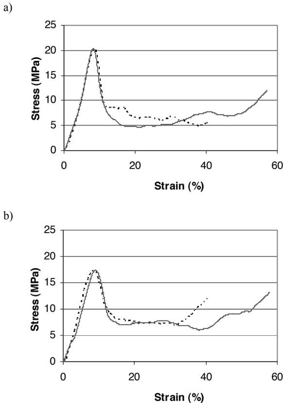
Fig. 11. Stress x strain curves in semi-static compression tests of AA7075/SiO<sub>2</sub>-MgO-Al<sub>2</sub>O<sub>3</sub> composites containing reinforcing particles with different sizes: (a) composite with fine vermiculite particles; (b) composite with coarse vermiculite particles. (Results for two different samples tested for each condition are shown. The tests represented by dotted lines were interrupted before onset of densification stage)
