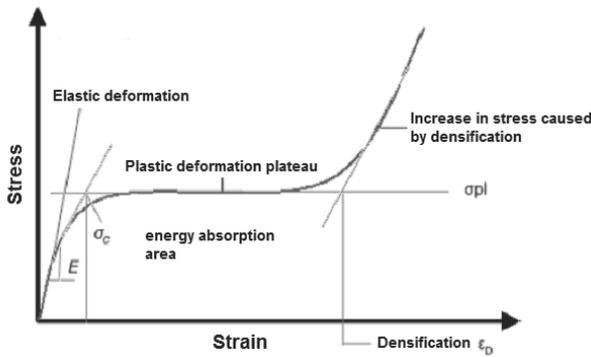
Fig. 10. Typical stress x strain curves of cellular metallic structures under compression
