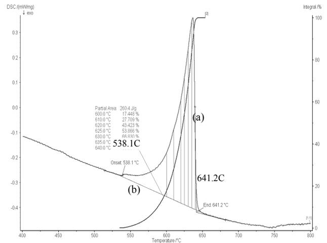
Fig. 2. Results of DSC tests for AA 7075 alloy. (a) energy variation x T; (b)  $f_l \times T$ . Heating cycle at 5 $^{\circ}$ C/min
