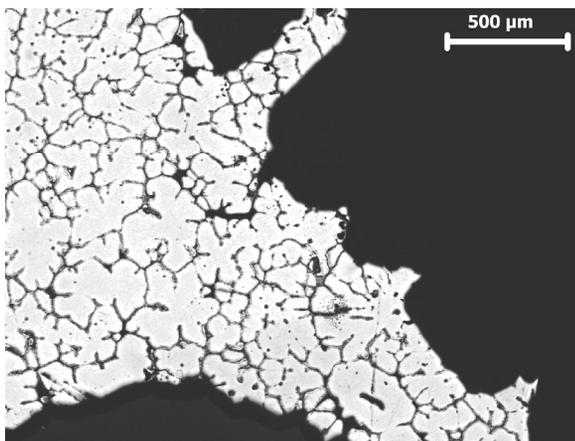
Fig. 8. Microstructure of the metallic matrix in the AA7075/SiO<sub>2</sub>-MgO-Al<sub>2</sub>O<sub>3</sub> composite produced. Optical microscopy
