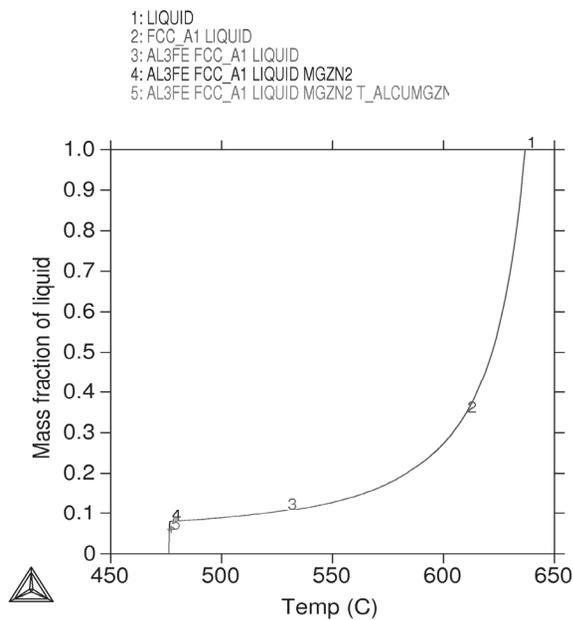
Fig. 3. Variation of  $f_l \times T$  for the AA 7075 alloy, according to thermodynamic calculations using a commercial package (Thermocalc<sup>R</sup>). Scheil condition
