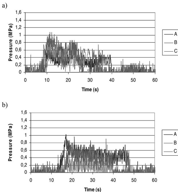
Fig. 4. Variation of  $P \times t$  during filling of pre-forms of: (a) fine; (b) coarse vermiculite particles. Three repetitions (A, B, C)
