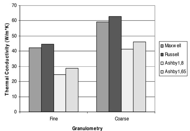
Fig. 12. Thermal conductivity of AA7075/SiO<sub>2</sub>-MgO-Al<sub>2</sub>O<sub>3</sub> composites, estimated by different theoretical models
