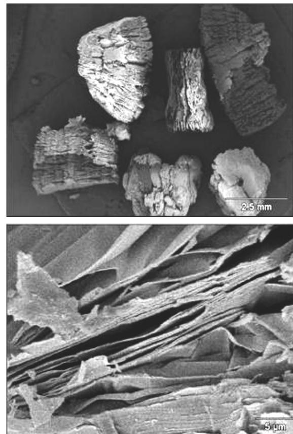
Fig. 1. General aspect of the expanded vermiculite particulates used as reinforcing material
