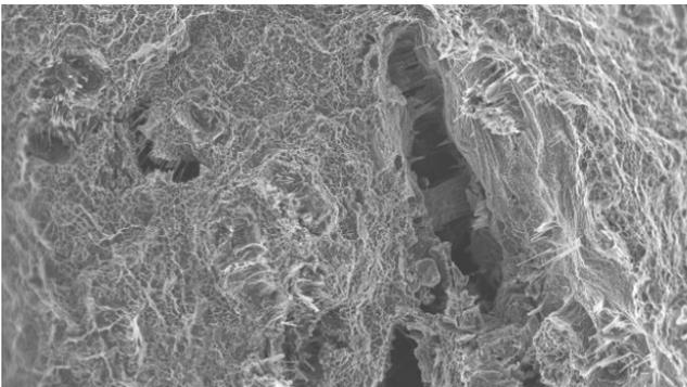
Fig. 10. Particular morphology of defects, pores and precipitates, observed on the fracture surface of sample type OP
