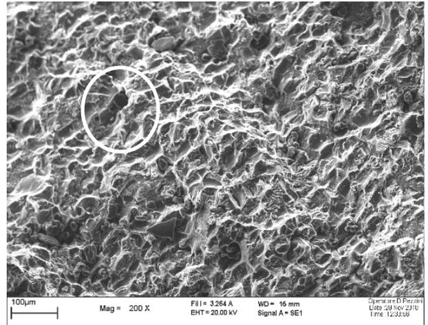
Fig. 4. SEM fracture surface of samples A showing the presence of the nanosized oxide inclusion
