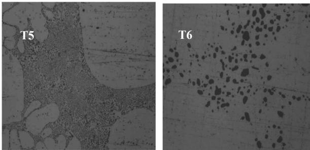
Fig. 3. Microstructure of T5 and T6 heat treated samples
