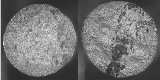
Fig. 9. Presence of defects, dark spots, distributed in preferential areas on the fracture surface of sample type OP
