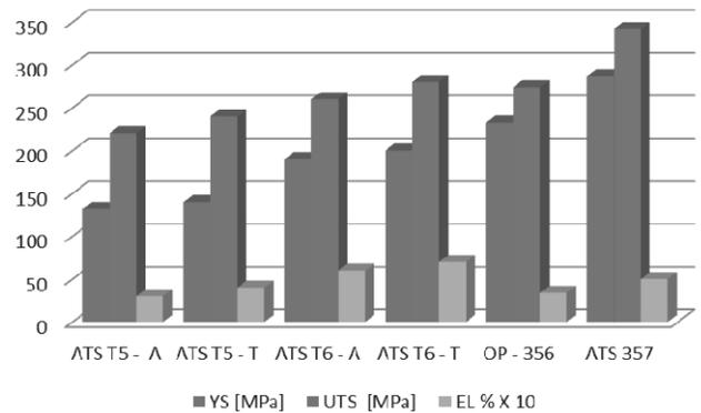
Fig. 7. Average tensile properties, Yield Strength (YS), Ultimate Tensile Strength (UTS) and ten times Elongation % of the different tested samples
