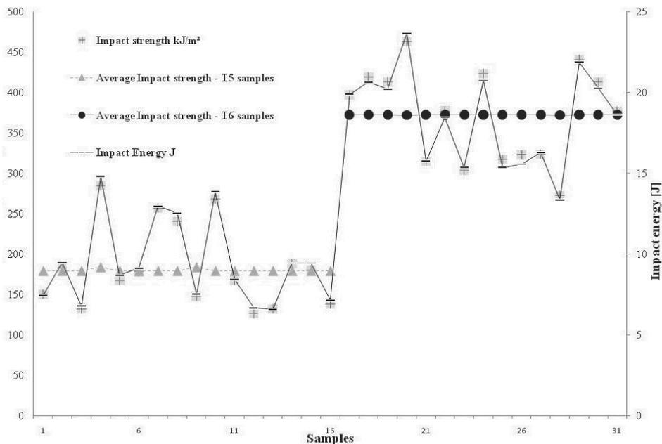
Fig. 5. Impact strength of the T5 and T6 heat treated samples in A356 alloy
