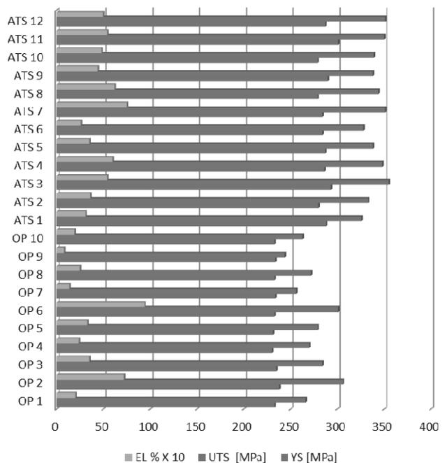
Fig. 8. Average tensile properties, Yield Strength (YS), Ultimate Tensile Strength (UTS) and ten times Elongation % of the different tested samples
