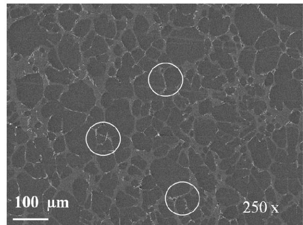
Fig. 2. Globular microstructure of  $\alpha$  aluminium solid solution
