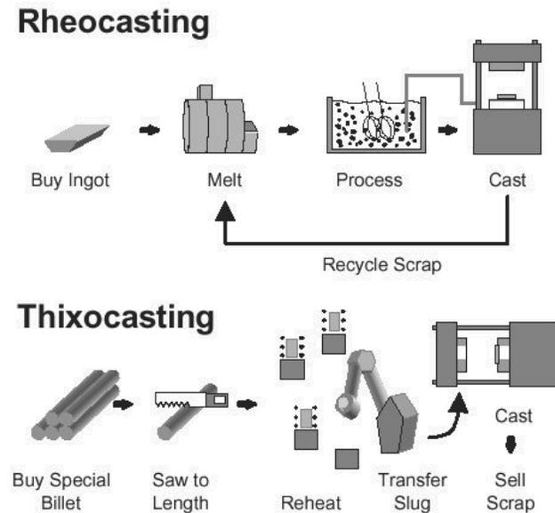
Fig. 1. distinctions between thixocasting and rheocasting
