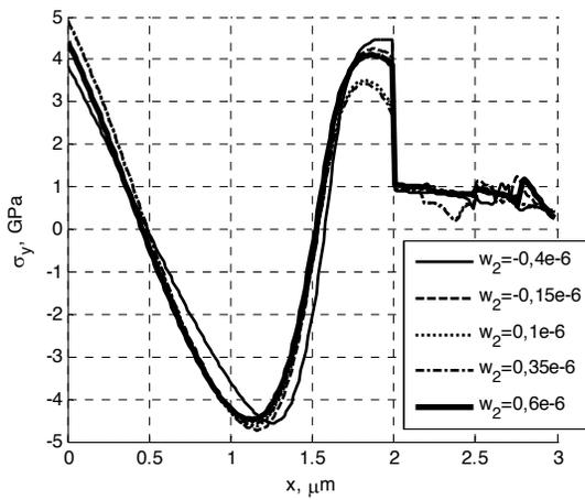
Fig. 9. Normal stresses  $\sigma_y$  as a function of  $x$  variable (distance from the surface), along Y1 comparative straight line for different values  $w_2$  for  $a_{1min}$ ,  $a_{2min}$   $w_{1min}$
