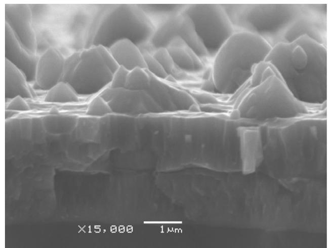
Fig. 1. Structure of TiAlN/TiN/Cr coating
