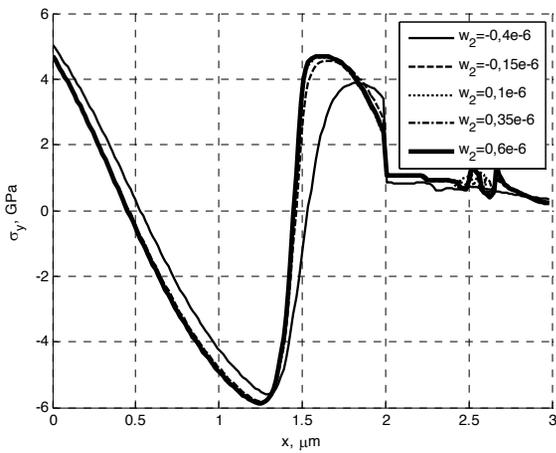
Fig. 17. Normal stresses  $\sigma_y$  as a function of  $x$  variable (distance from the surface), along Y1 comparative straight line for different values  $w_2$  for  $a_{1max}$ ,  $a_{2min}$  and  $w_{1min}$
