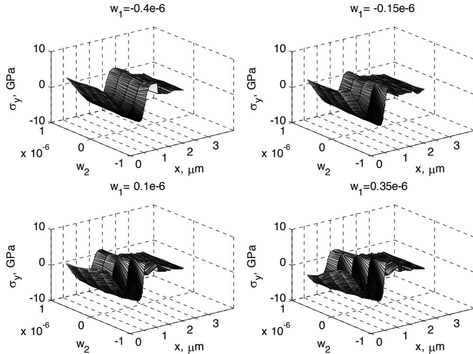
Fig. 22. Normal stresses  $\sigma_y$  as a function of  $x$  variable (distance from the surface), along Y1 comparative straight line for different values  $w_1$  and  $w_2$  for  $a_{1min}, a_{2max}$
