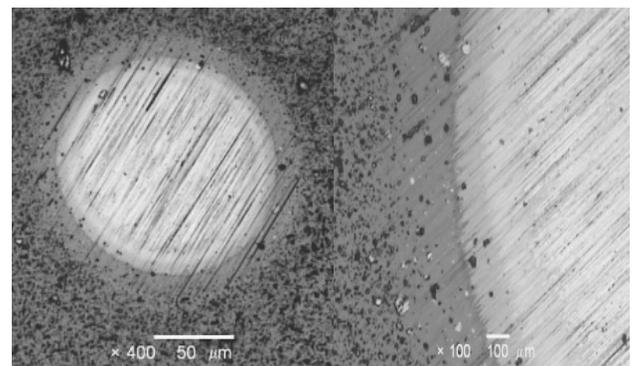
Fig. 2. TiAlN/TiN coating with gradient transition layer
