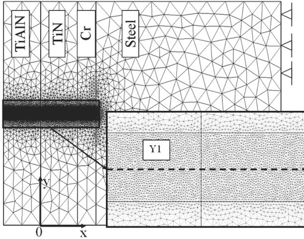
Fig. 3. The schema of the modelled object with mesh
