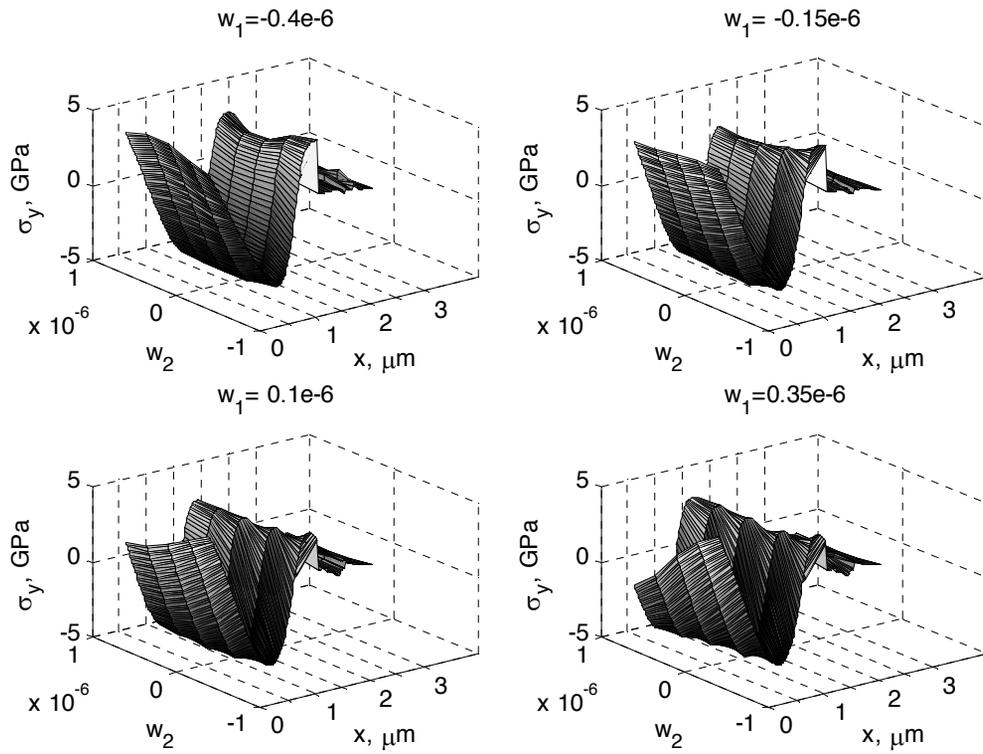
Fig. 21. Normal stresses  $\sigma_y$  as a function of  $x$  variable (distance from the surface), along Y1 comparative straight line for different values  $w_1$  and  $w_2$  for  $a_{1min}, a_{2min}$
