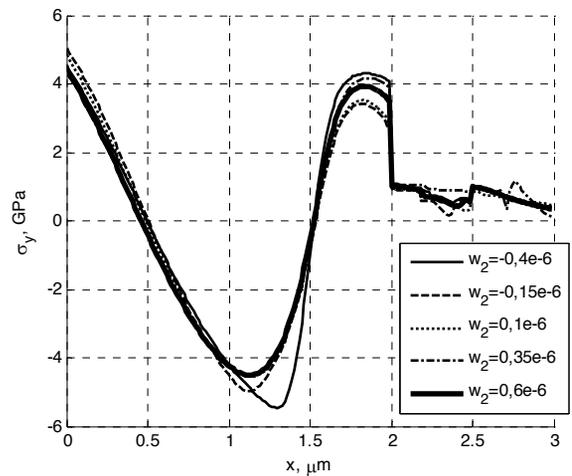
Fig. 13. Normal stresses  $\sigma_y$  as a function of  $x$  variable (distance from the surface), along Y1 comparative straight line for different values  $w_2$  for  $a_{1min}$ ,  $a_{2max}$   $w_{1min}$
