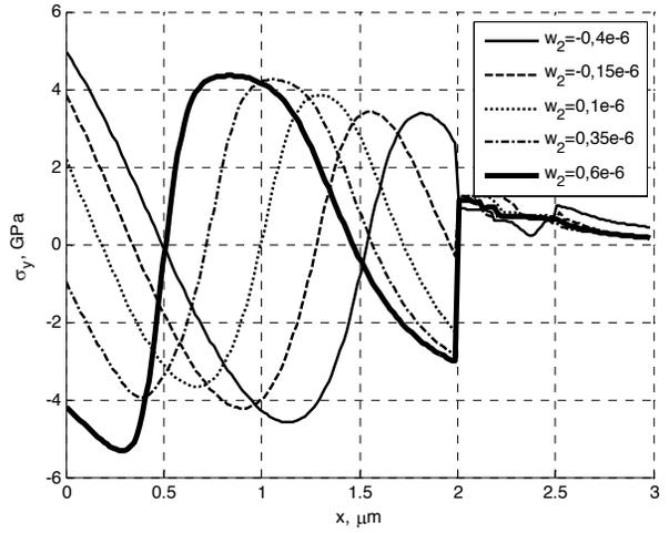
Fig. 18. Normal stresses  $\sigma_y$  as a function of  $x$  variable (distance from the surface), along Y1 comparative straight line for different values  $w_2$  for  $a_{1max}$ ,  $a_{2min}$  and  $w_{1max}$
