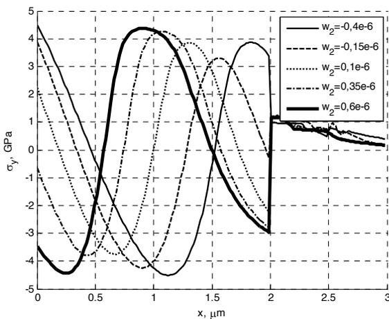
Fig. 11. Normal stresses  $\sigma_y$  as a function of  $x$  variable (distance from the surface), along Y1 comparative straight line for different values  $w_2$  for  $a_{1min}$ ,  $a_{2min}$   $w_{1max}$
