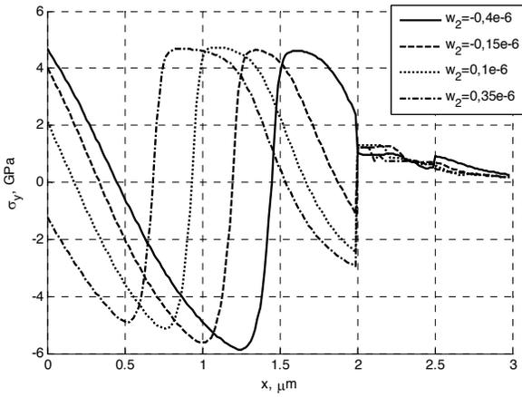
Fig. 15. Normal stresses  $\sigma_y$  as a function of  $x$  variable (distance from the surface), along Y1 comparative straight line for different values  $w_2$  for  $a_{1min}$ ,  $a_{2max}$   $w_{1max}$
