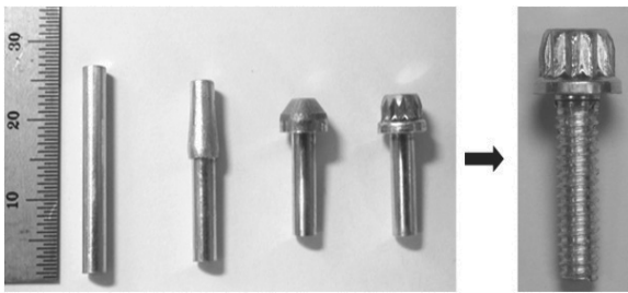
Fig. 5. The aluminum bolt manufactured by the ultra-fine grained specimen [44]
