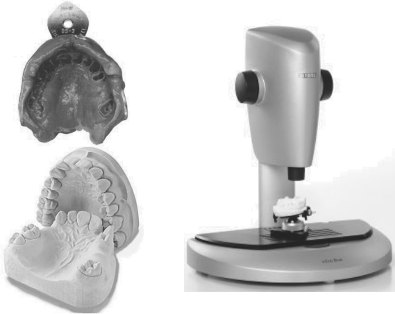
Fig. 2. Dental impression, gypsum models and extra oral 3D digitization system Sirona "InEos Blue"
