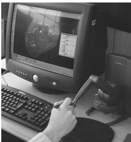
Fig. 8. Virtual sculpting system with haptic arm
