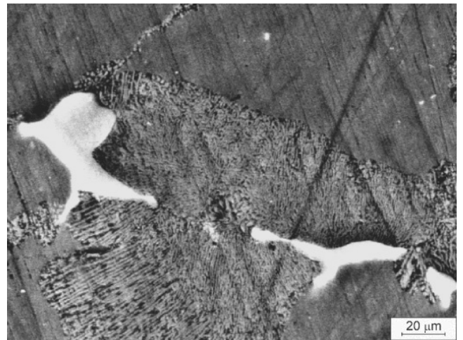
Fig. 2. Structure of the MCMgAl9Zn1 alloy after aging at the temperature of 190°C for 15 hours
