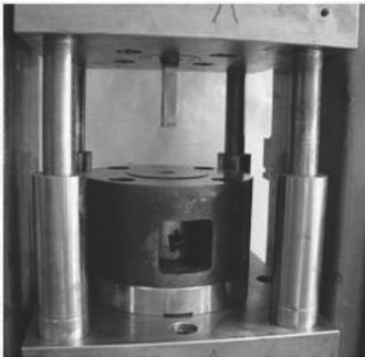
Fig. 15. Press DP 1600 kN with the ECAP tool, a) general view, b) detail of the forming tool
