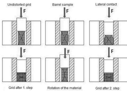
Fig. 3. Schematic illustration of the CCDC method
