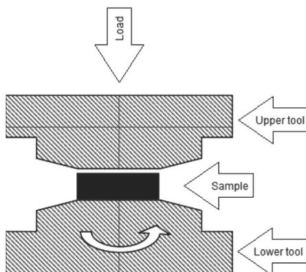
Fig. 1. Schematic illustration of the HPT method
