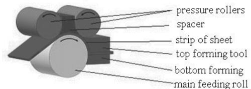
Fig. 14. Scheme of the DRECE method
