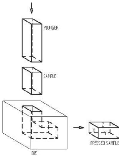
Fig. 7. Schematic illustration of the ECAP method
