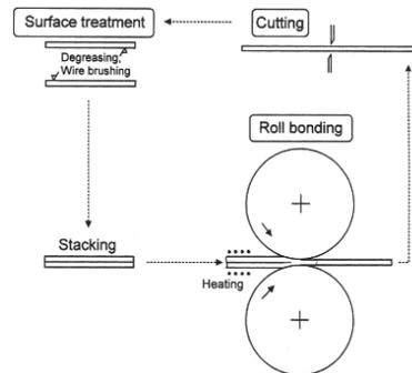
Fig. 5. Schematic illustration of the ARB method
