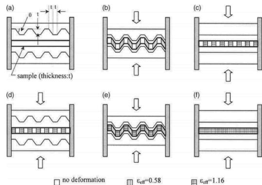
Fig. 6. Schematic illustration of the CGP method
