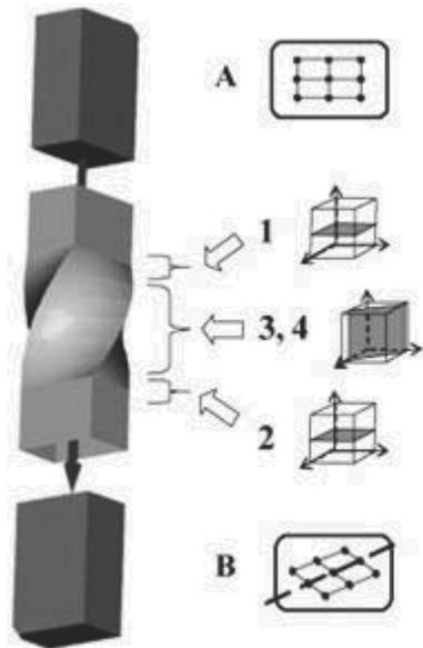
Fig. 11. Principle of the Twist Extrusion Process
