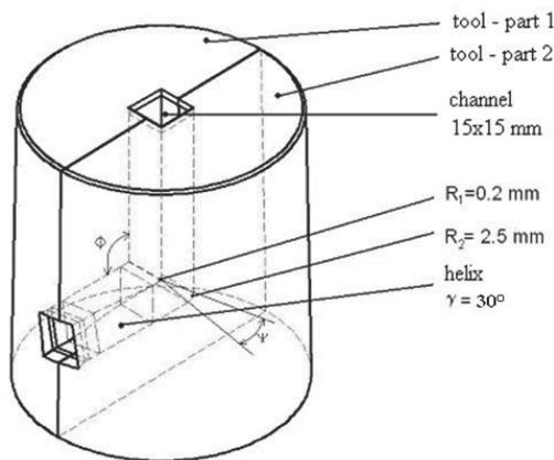
Fig. 12. Insert of the ECAP tool with built-in helix
