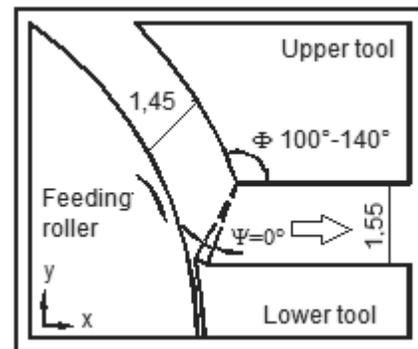
Fig. 10. Angle of the channel  $\Phi$
