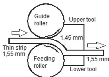
Fig. 9. Schematic illustration of the DCAP method
