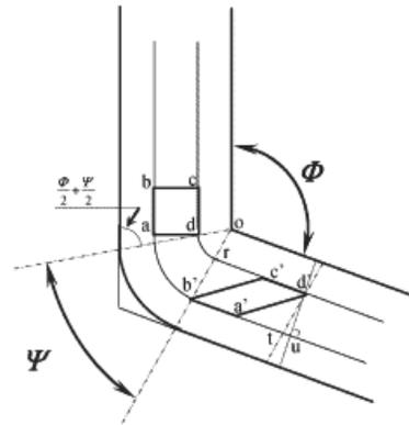
Fig. 8. Dependence on the angle  $\Psi$  of the arc of curvature
