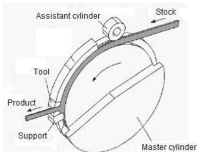
Fig. 4. Schematic illustration of the Conform method
