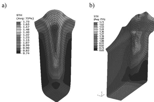
Fig. 4. Thickness distribution for optimized plans for a) Square Box and b) Rectangular Box (Adapted from Abdelmaguid et al., 2012)
