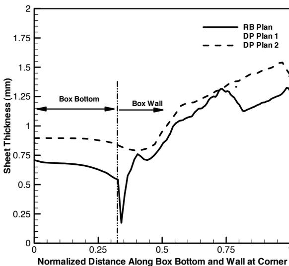
Fig. 5. Thickness distribution along the bottom of and wall of rectangular box. (After Abdelmaguid et al. [46])
