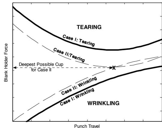
Fig. 1. BHF Working Window (After Gharib *et al.* [12])
