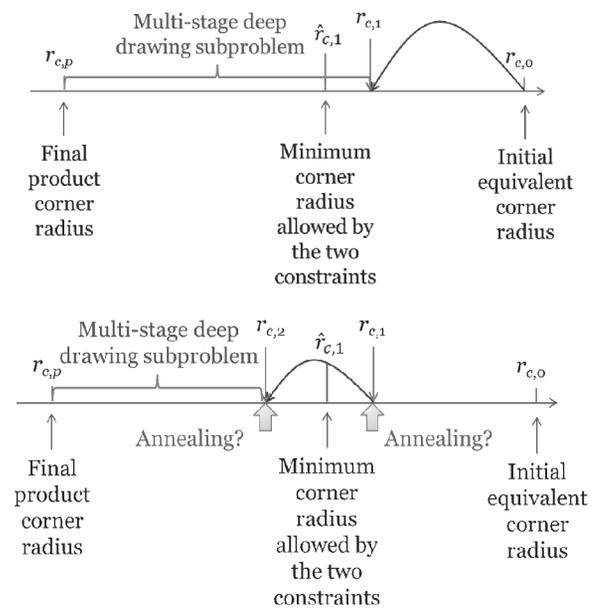
Fig. 3. An illustration of sub-problems generation
