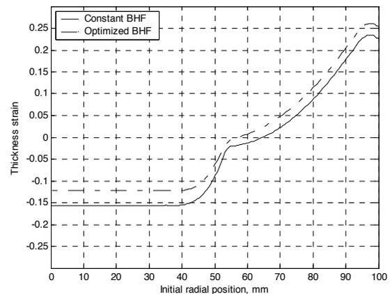
Fig. 2. Thickness strain distributions for the constant BHF and optimized BHF (After Gharib *et al.* [12])
