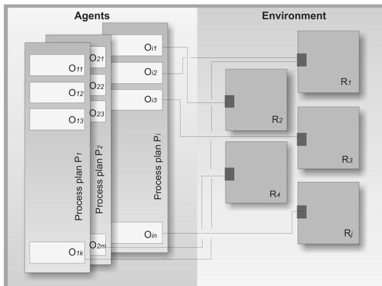
Fig. 1. Process plans as sets of agents **O** operating in the environment composed of resources **R**
