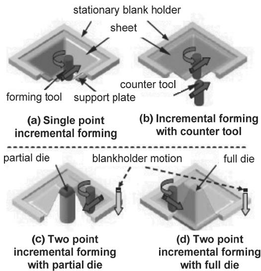
Fig. 2. Classification of sheet incremental forming
