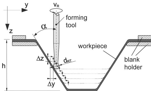
Fig. 1. Basic principle of incremental forming
