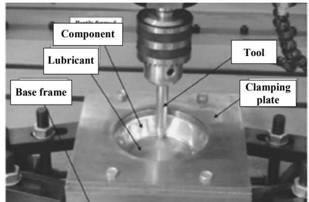
Fig. 8. The CNC milling machine with the tool setup applied during the experiments
