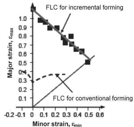
Fig. 4. Forming Limit Diagrams for conventional and incremental sheet metal forming
