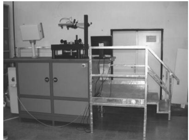
Fig. 9. The universal formability testing machine with the Vialux optical strain measurement device
