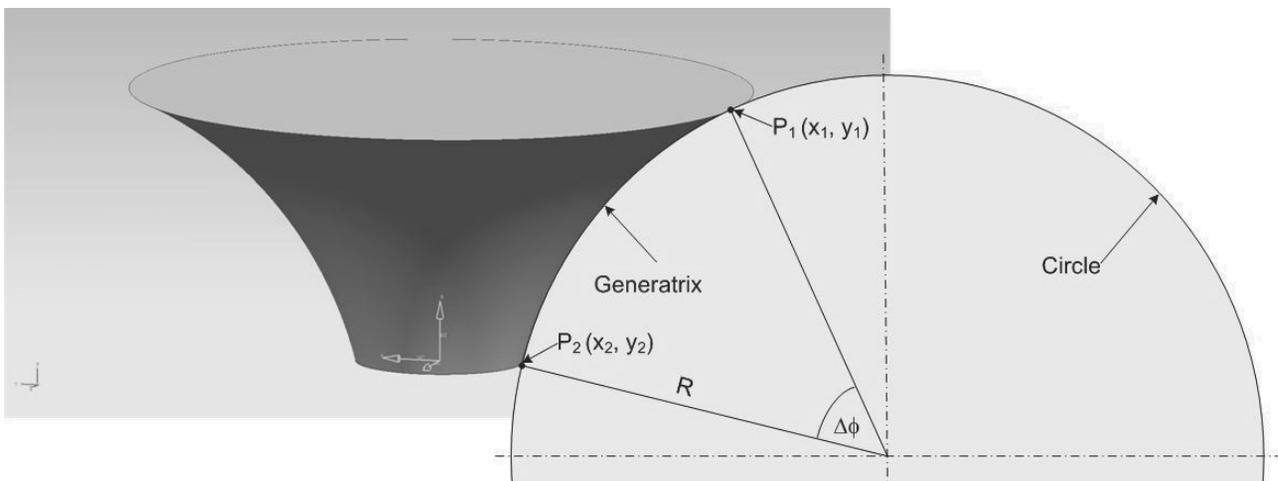
Fig. 6. Illustration of a circular generatrix derivatio
