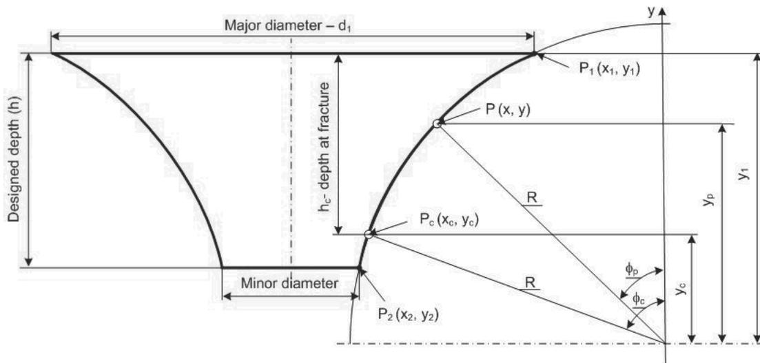
Fig. 7. Principle scheme for the calculation of limit draw angle and the limit thinning
