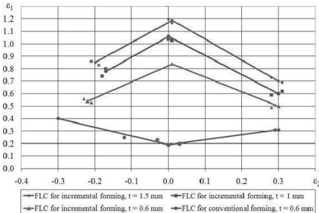
Fig. 10. Comparison of FLDs for incremental and conventional sheet forming (Material grade: Al 1050-A)
