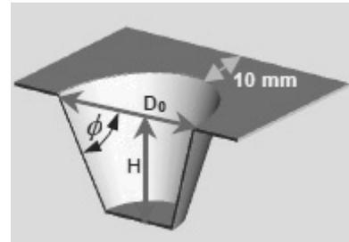
Fig. 3. Benchmark specimen to determine the limit draw angle
