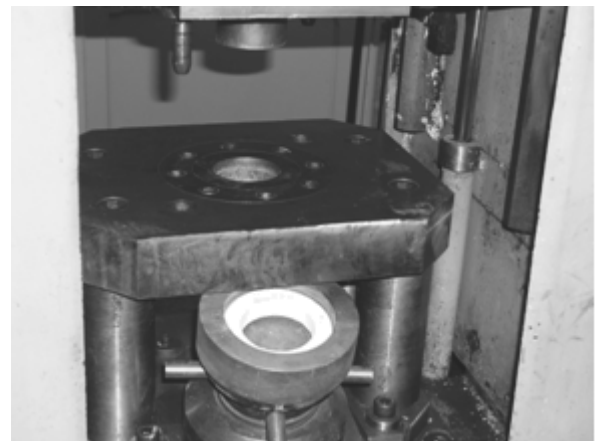
Fig. 2. Mould for squeeze casting with fibre preform before closing
