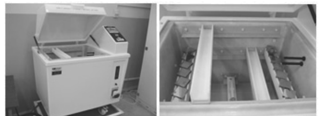
Fig. 3. SF/200-A salt spray cabin [22]
