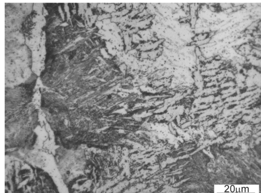
Fig. 1. Microstructure of the 38MnCrNi6-4-4 steel after re forging. Hardness 205 HV30. Etched by 3% nital
