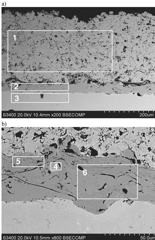
Fig. 4. Microstructure of thermal barrier coating with calcium-stabilised zirconium oxide ceramic layer (METCO 201) (a) and detailed construction of the MeCrAlY-type interlayer (b) with indicated spots for chemical composition analysis
