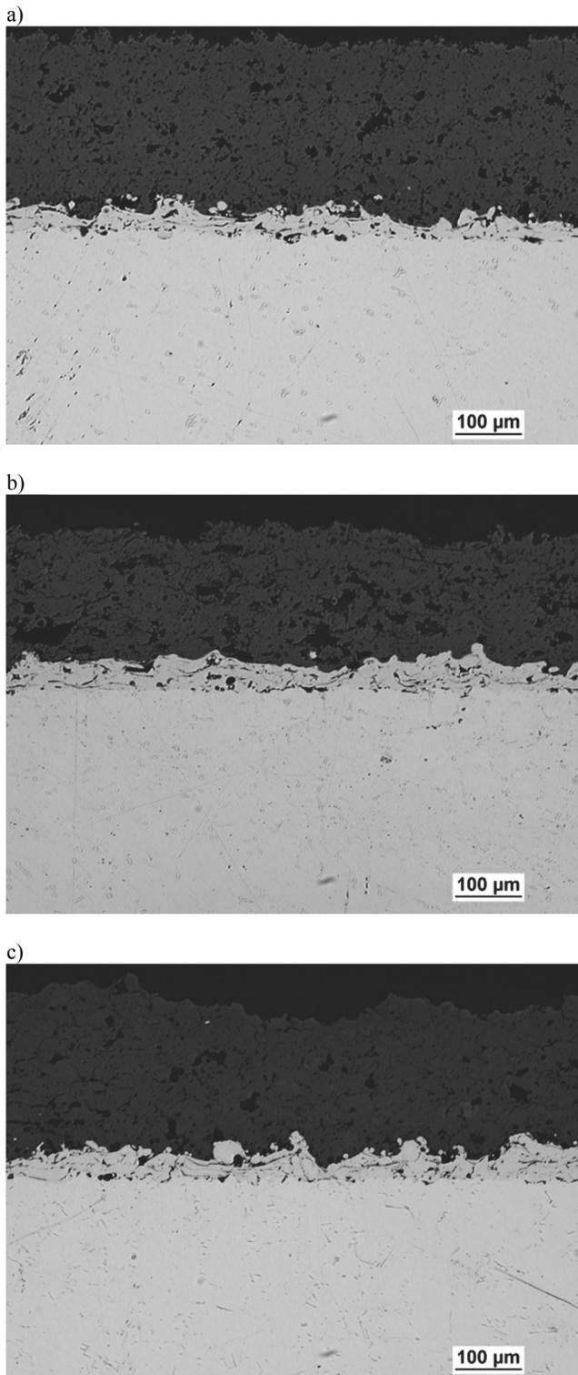
Fig. 2. Microstructure of thermal barrier coating obtained by the APS method with the use of calcium-stabilised (a) yttrium-stabilised (b) and magnesium-stabilised (c) zirconium oxides in the ceramic layer
