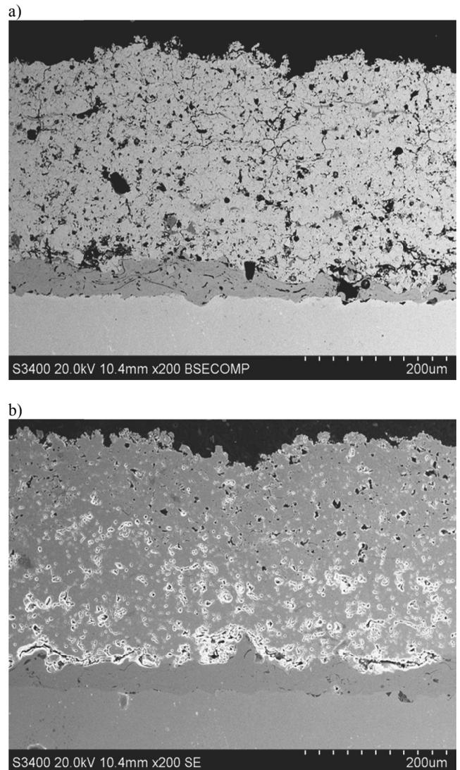
Fig. 3. Microstructure of thermal barrier coating with calcium-stabilized zirconium oxide ceramic layer (METCO 201)
