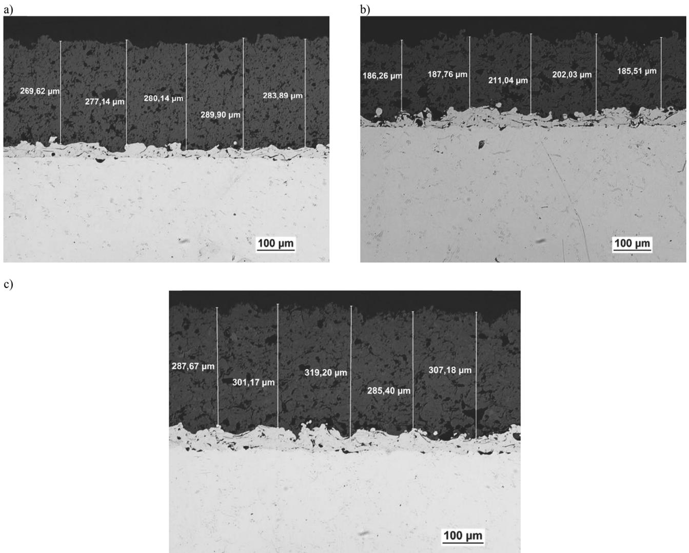
Fig. 1. Thickness measurement of thermal barrier coating obtained by the APS method with the use of calcium-stabilised (a) yttrium-stabilised (b) and magnesium-stabilised (c) zirconium oxides in the ceramic layer.
