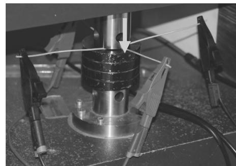
Fig. 1. Electrical contact resistance measurement - Kelvin method
